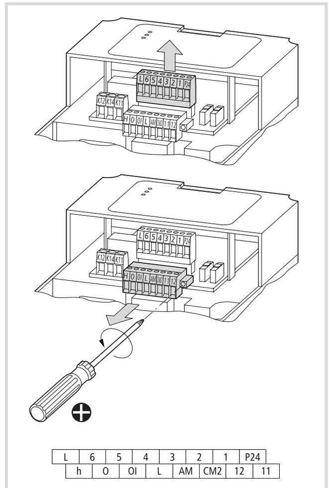
Figure 8: Position of control signal terminals
