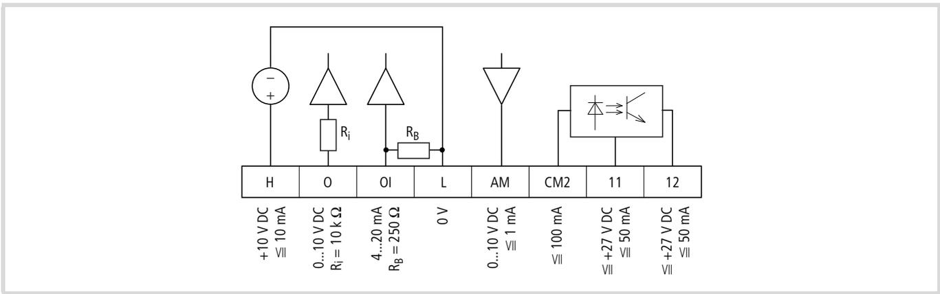
Figure 11: Lower control signal terminal bank
