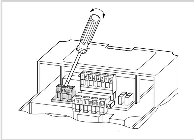
Figure 7: Position signalling relay terminals
