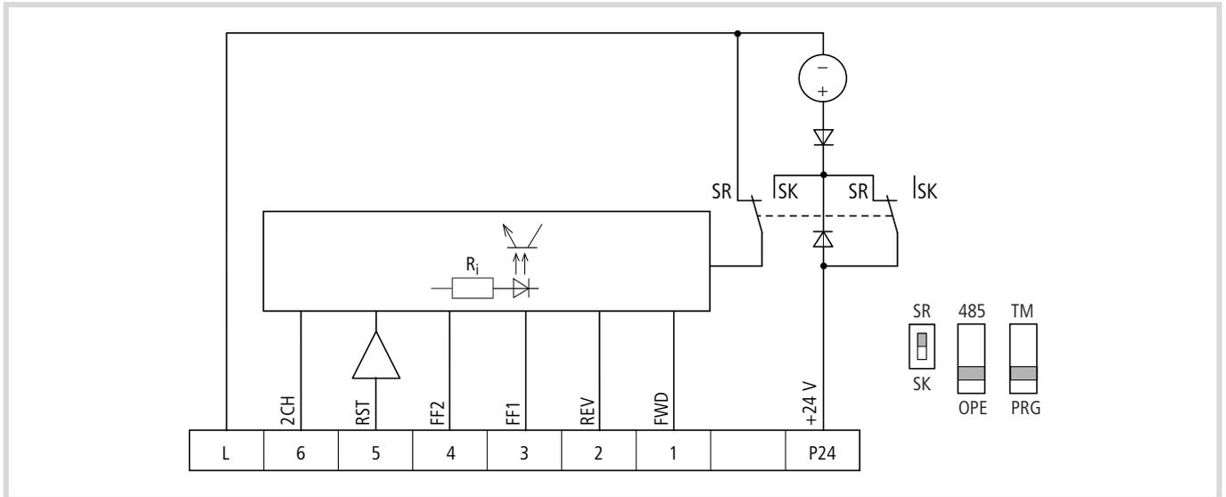
Figure 9: Upper control signal terminal bank
