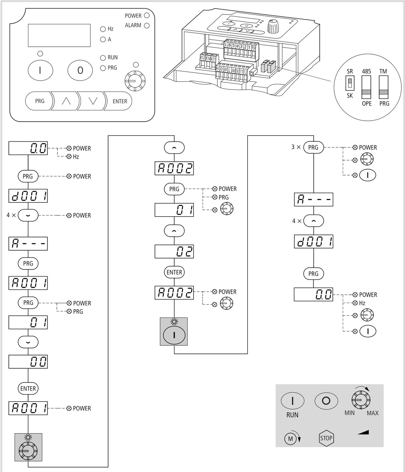
Figure 27: Reference values and control signals via keypad
