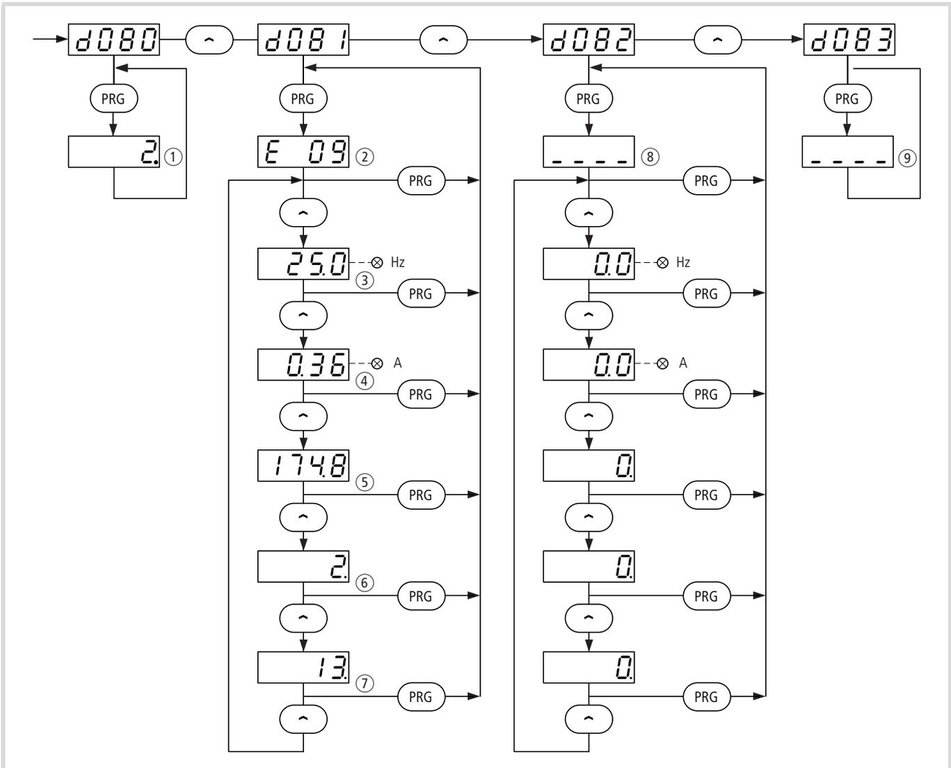
Figure 28: Data in the fault register at the time of the fault signal
