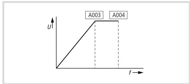
Figure 25: End frequency 60 Hz
