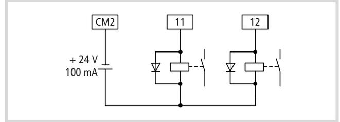
Figure 13: Relay with freewheeling diode (for example ETS-VS3)
