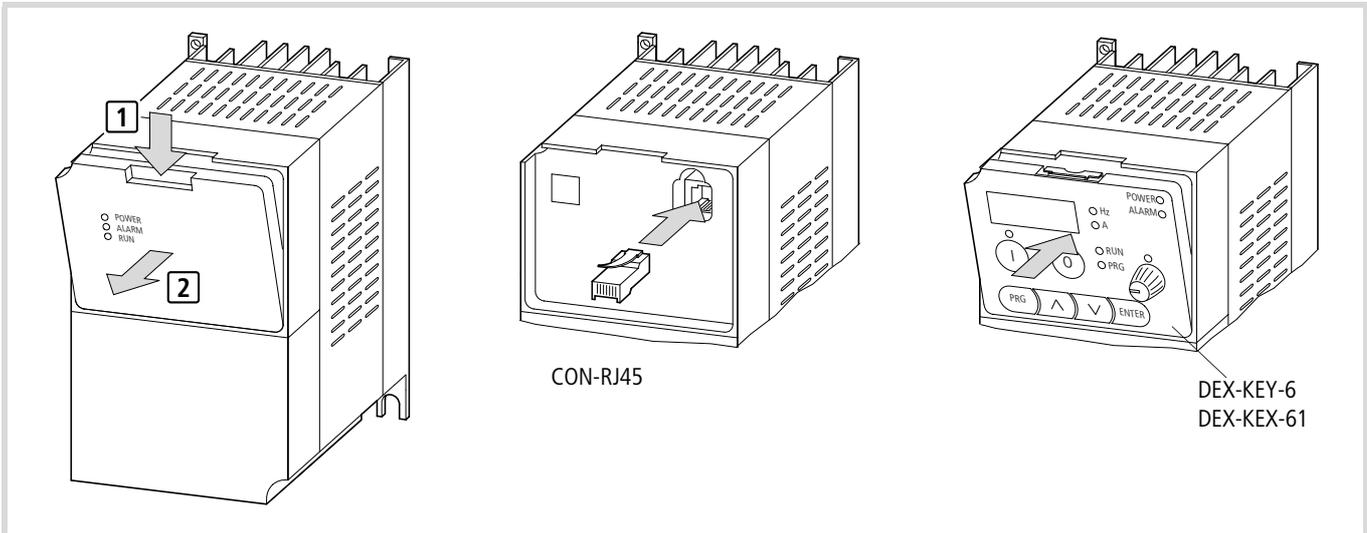
Figure 21: Fitting keypad DEX-KEY-6... in DF51
