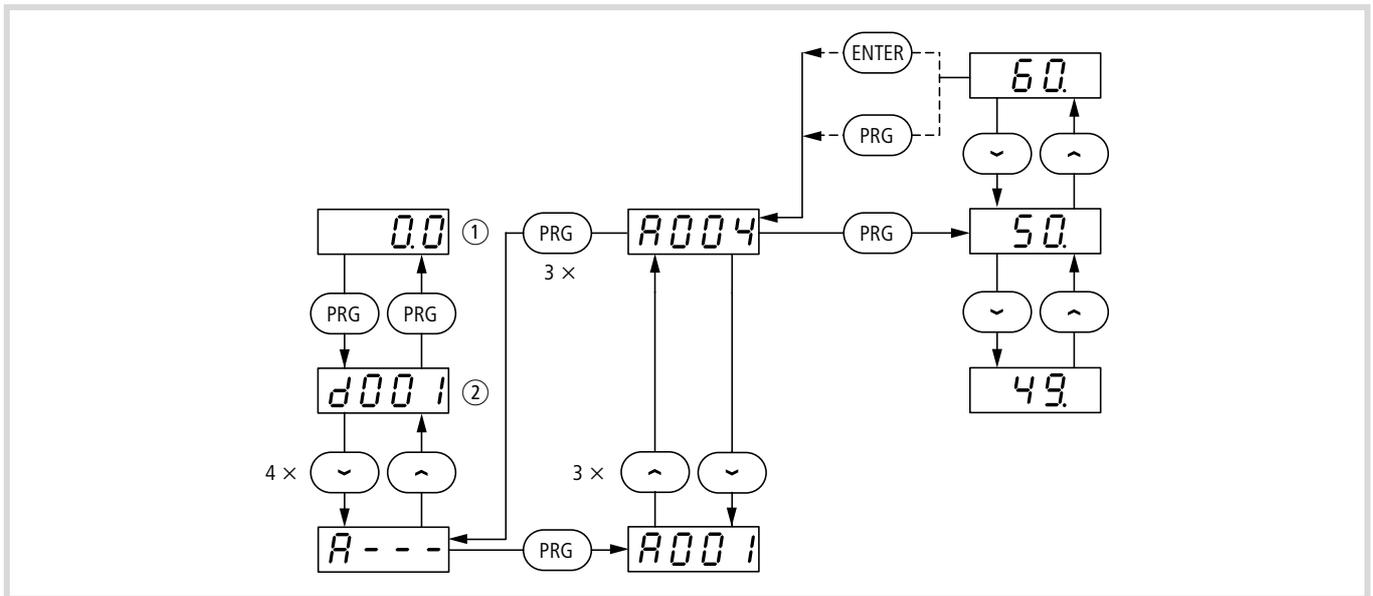
Figure 26: Change end frequency (example with default setting)
