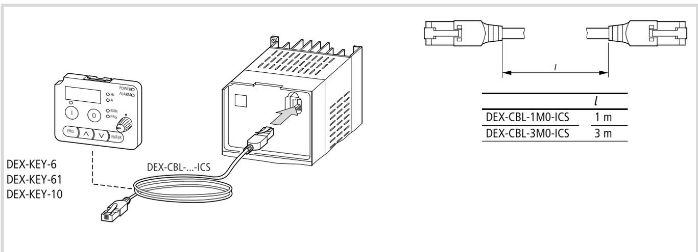
Figure 22: Frequency inverter with connection cable DEX-CBL-...-ICS
