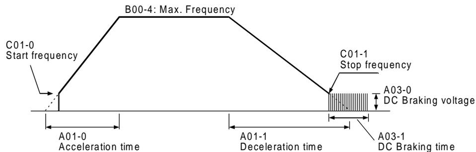
This is the acceleration/deceleration ramp time validated during normal use (when sequence command CSEL is OFF). The inverter may trip if the set time is too short.
