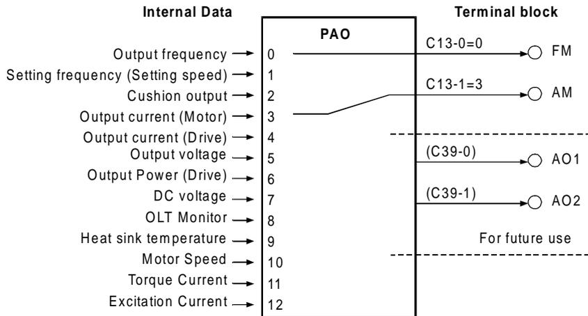
Fig. 5-8 Analog output assignment
