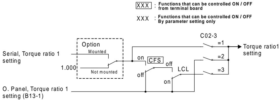
Fig. 5-14 Torque ratio 1 setting selection
