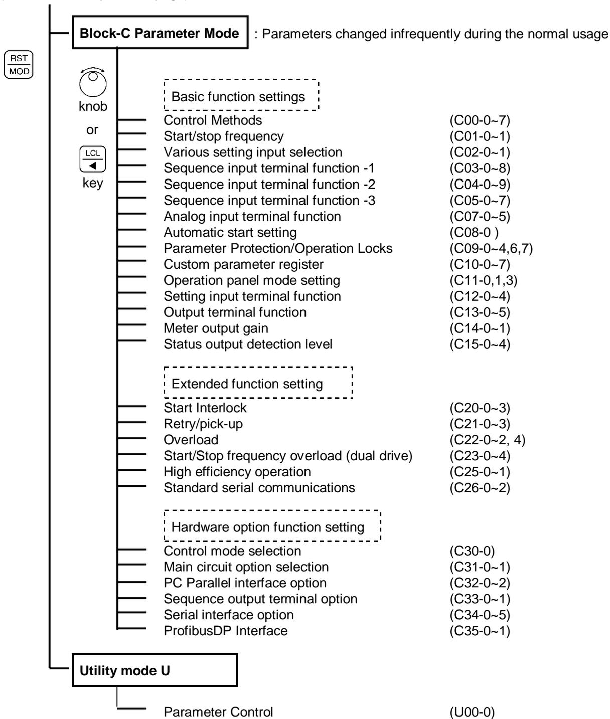
**(Note)** At the default setting, only the basic functions are displayed, but the extended function, software option function, hardware option function parameters are skipped. Thus, to display these parameters, change parameter A05-0 to 3 (parameter B, C block skip setting), so that the target parameters are displayed.
