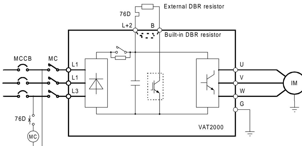
**Fig. 7-3 DBR circuit**
