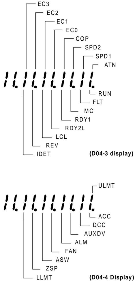
Fig. 5-6 Sequence output monitor
