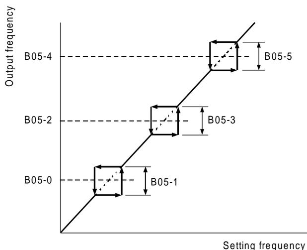
**(Note)** This function controls the frequency setting, so the above skip frequency area will be passed with a ramp function.
