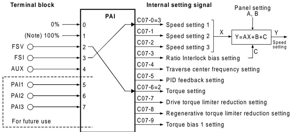
(Note) The torque setting is 300% when C07-6 is 1.
