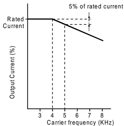
**Fig. 1-4 Derating according to carrier frequency for drives larger than U2KX45K0S**
