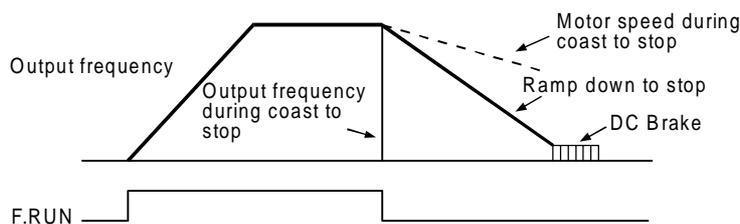
**(Note)** To restart after coast to stop, confirm that the motor has stopped. The inverter may trip if attempted when the motor is running. (For V/f control)
