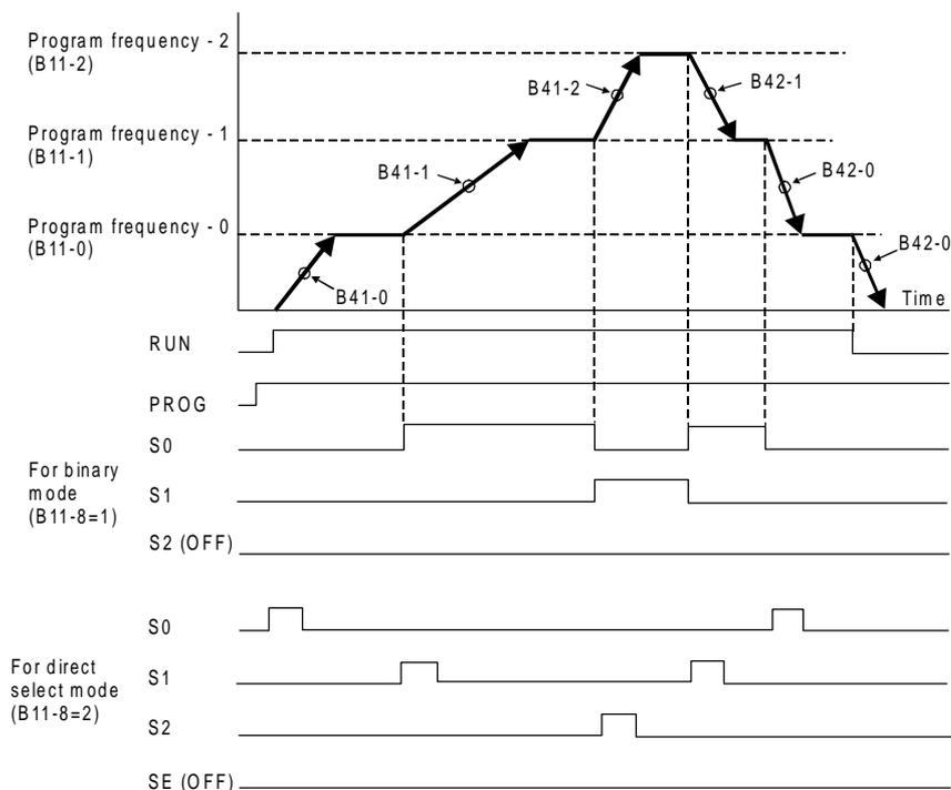
**(Note)** The acceleration/deceleration ramp time-2 (B10-0, 1) will be selected by turning the sequence command CSEL ON even when using the program ramp (B40-0=2).
