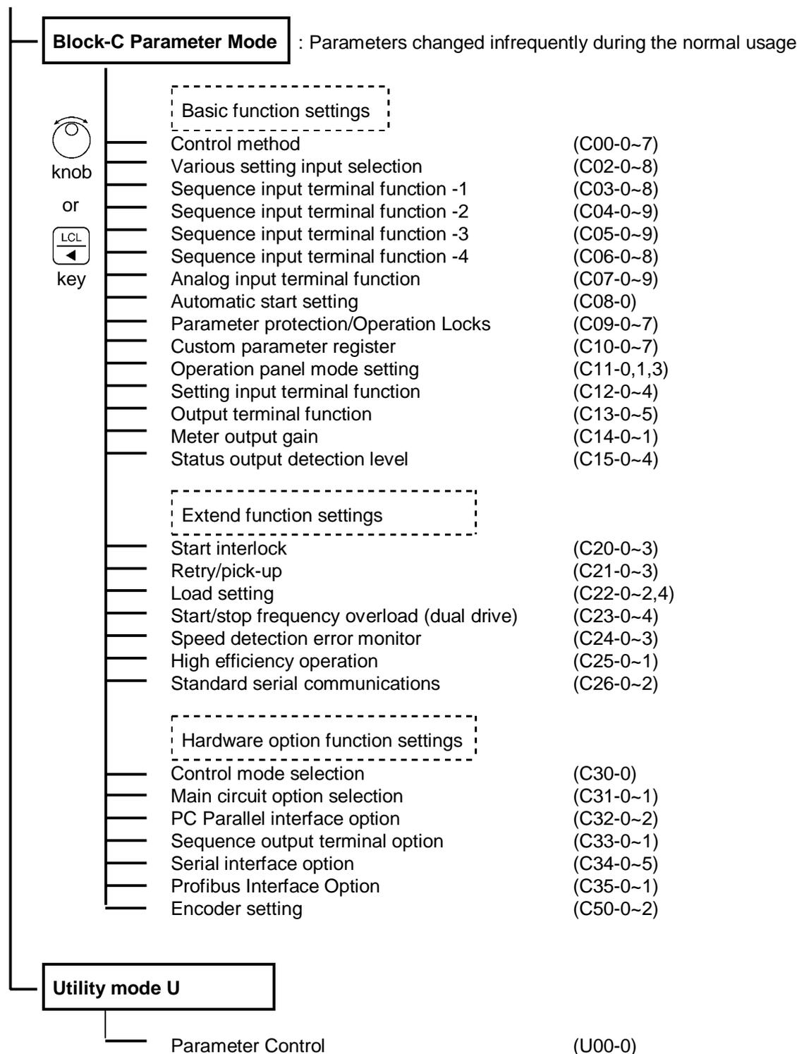
**(Note)** At the default setting, only the basic functions are displayed. The extended function, software option function, hardware option function parameters are skipped. Thus, to change these parameters, change parameter A05-0 to 3 (parameter B, C block skip setting), so that the target parameters are displayed.
