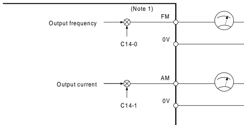
**(Note 1)** The maximum output voltage of the FM and AM outputs is approx. 11V. If a large value is set in C14-0 and 1, a voltage exceeding 11V will not be output.
