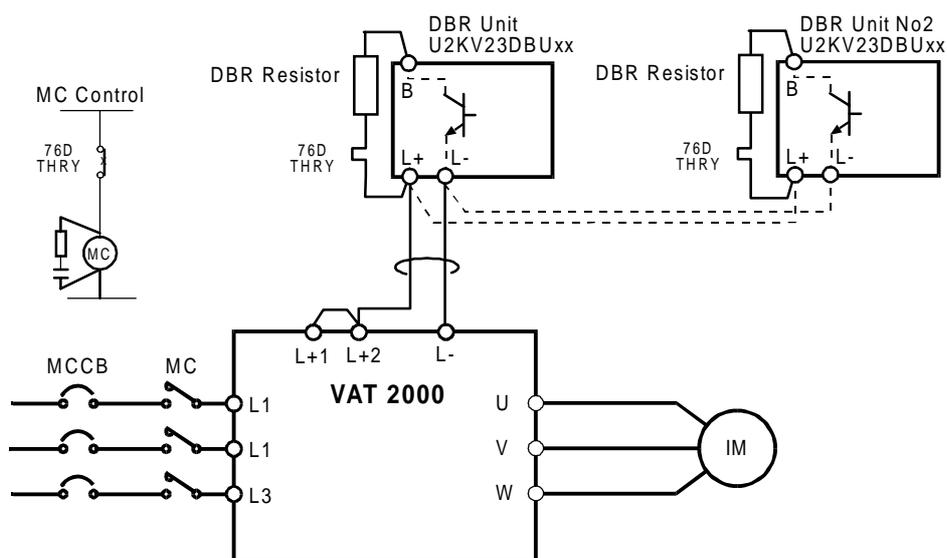
**Fig. 7-4 DBR connection**
