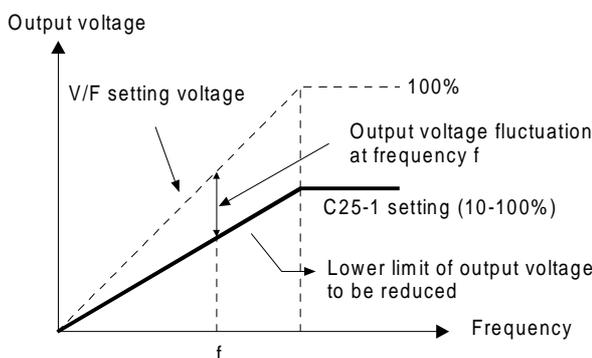
**high-efficiency operation principle**
