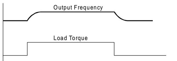
**(Note 1)** The slip compensation will not function in respect to the regenerative torque.
