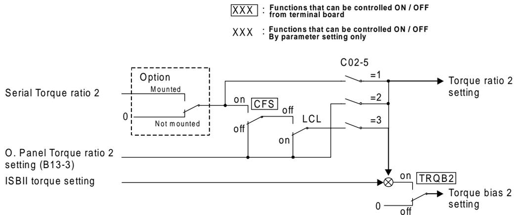
Fig. 5-15 Torque ratio 2 setting selection
