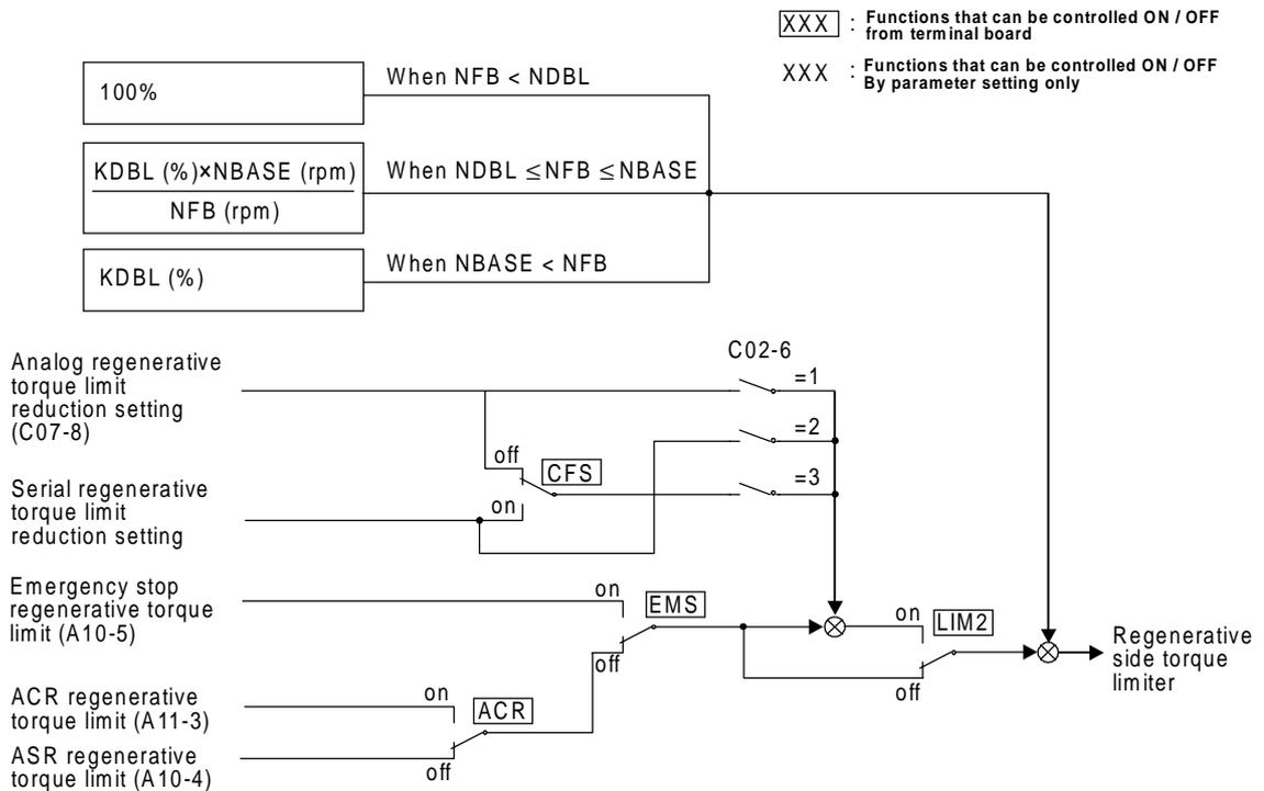
Fig. 5-13 Regenerative torque limit setting selection
