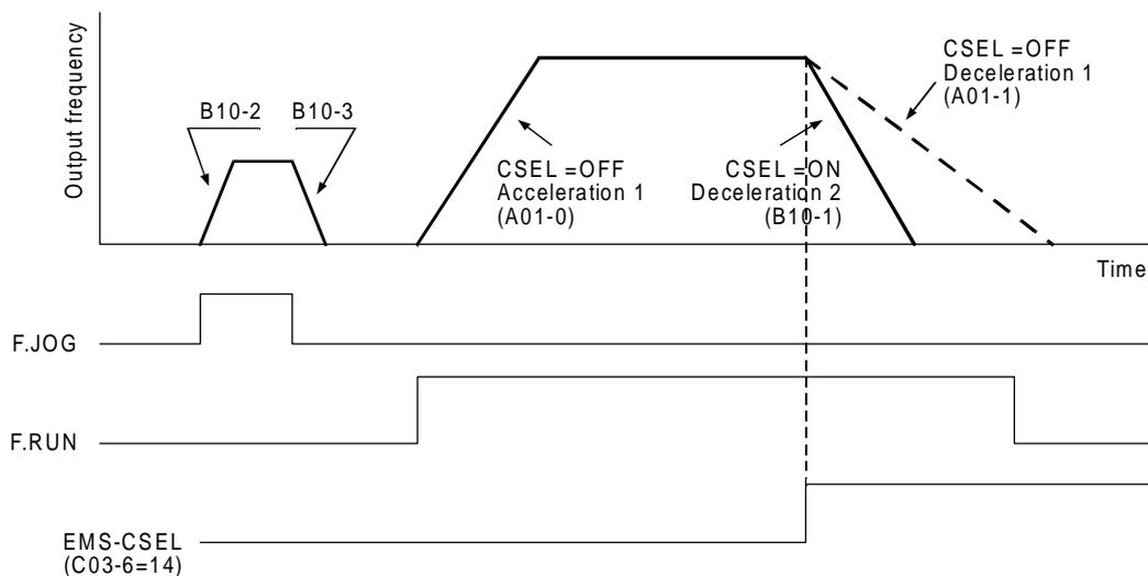
The above run example shows the case when the sequence command CSEL is connected to the EMS terminal (C03-6=14), and the run is decelerated with ramp down time -2 during emergency stop.
