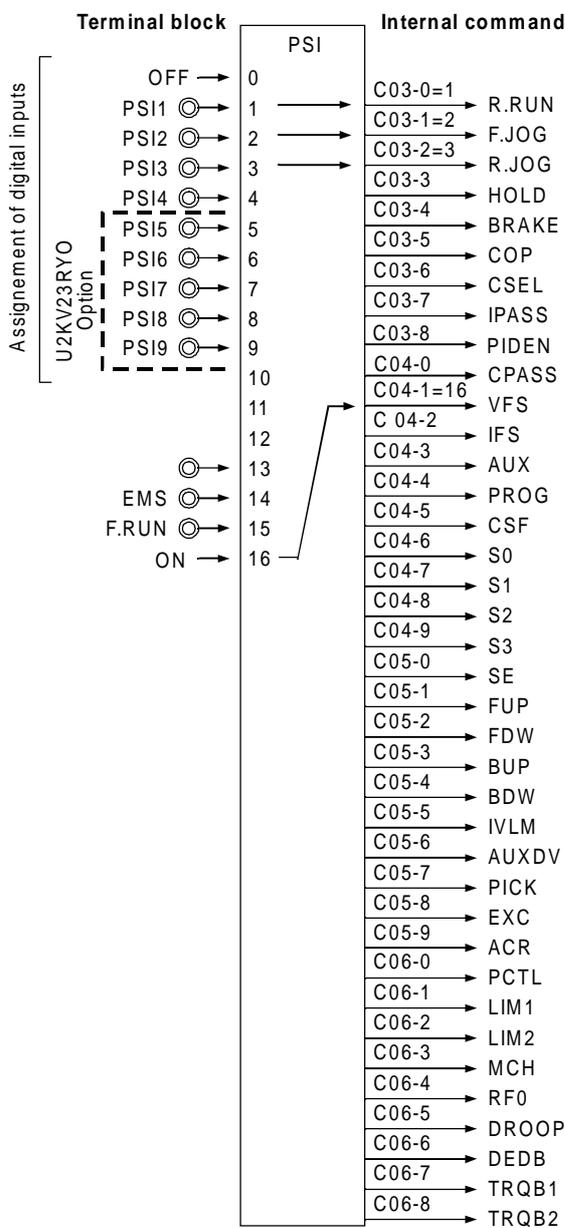
Fig. 5-3 Assignment of sequence input
