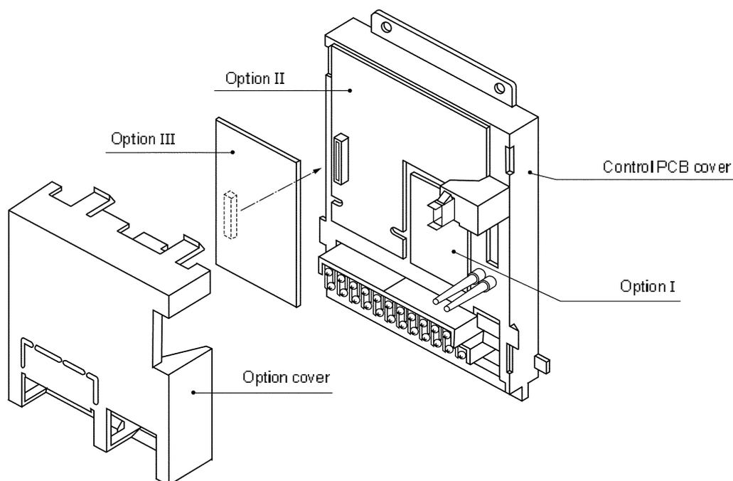
**Built-in PCB option mounting drawing**
