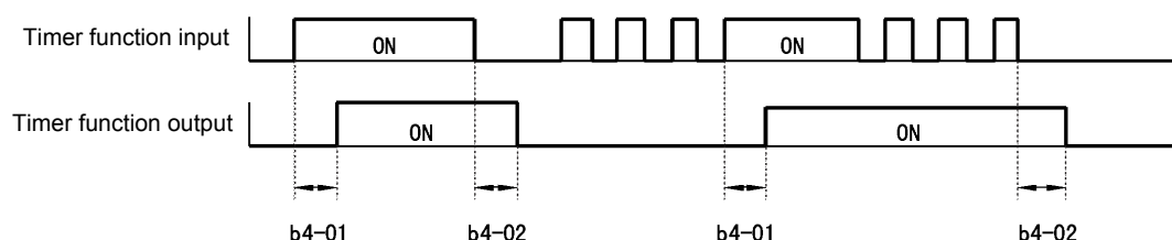
Fig 6.56 Timer Function Operation Example
