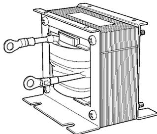
The DC Reactor suppresses harmonic current generated from the Inverter and improves the power factor of the Inverter. The DC Reactor suppresses harmonic current more effectively than the AC Reactor. Furthermore, the DC Reactor can be used in combination with the AC Reactor.
