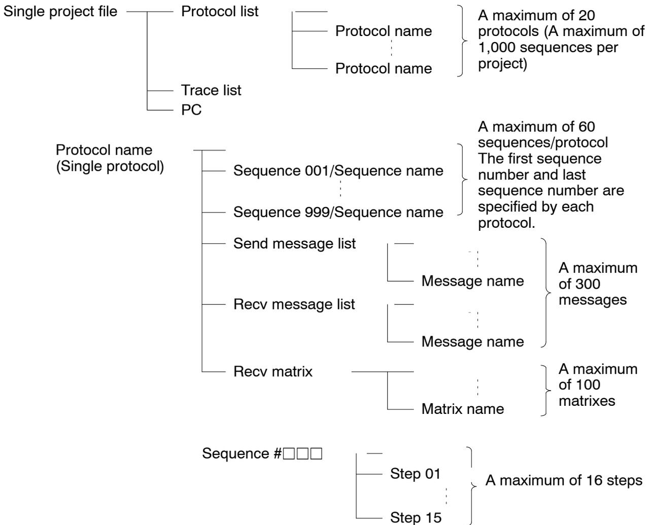
**Note** The standard system protocol incorporated by the Communications Board cannot be edited or transferred. To make use of the standard system protocol, copy it to the project file and edit it.
