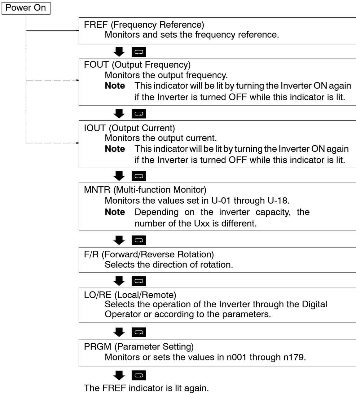
**Note** The setting unit of the frequency reference and output frequency is determined by the set value in n035. The default unit is Hz.
