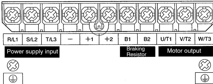
**Note** For single-phase input, connect R/L1 and S/L2.
