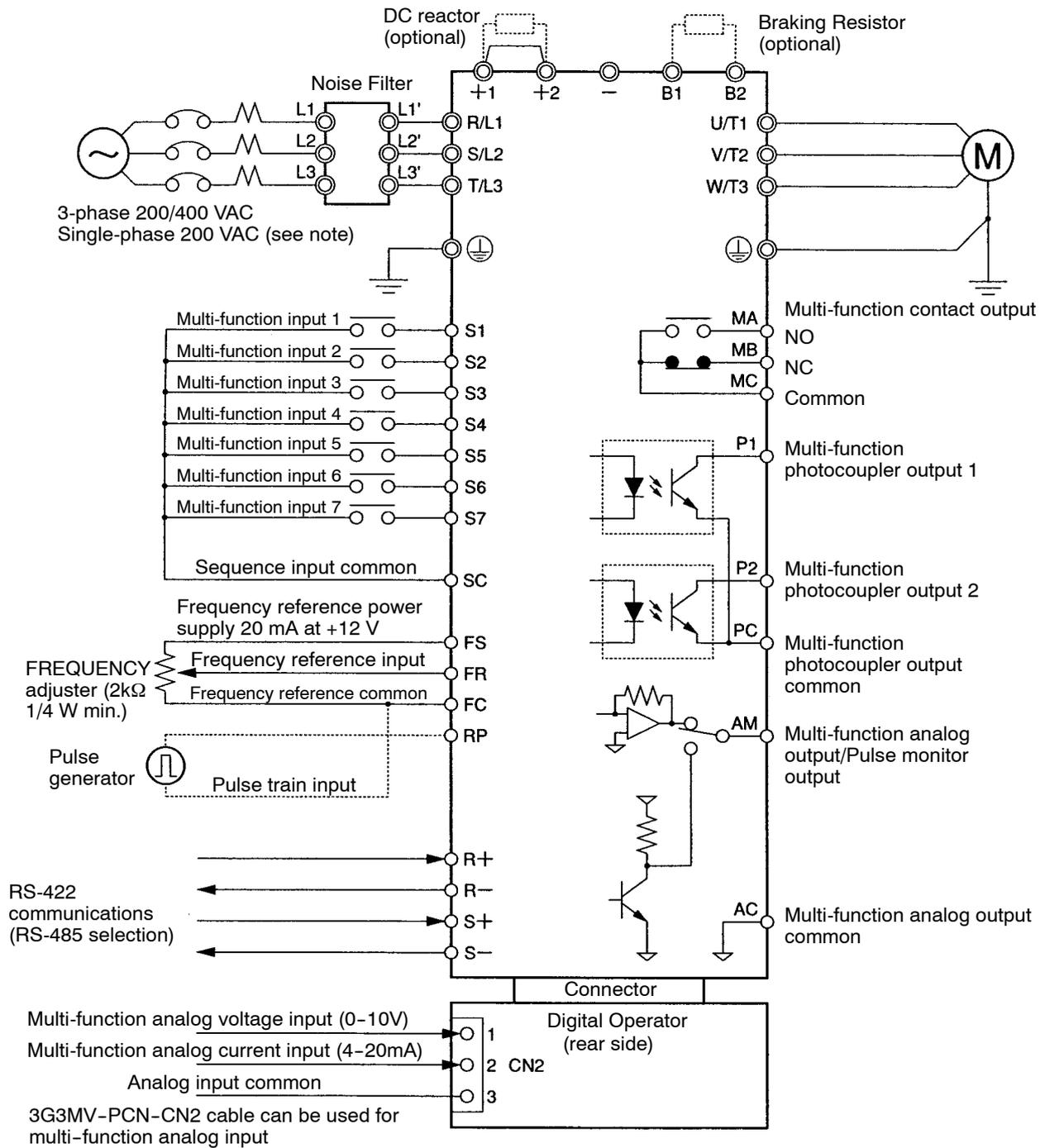
**Note** Connect single-phase 200 VAC to terminals R/L1 and S/L2 of the 3G3MV-AB□.
