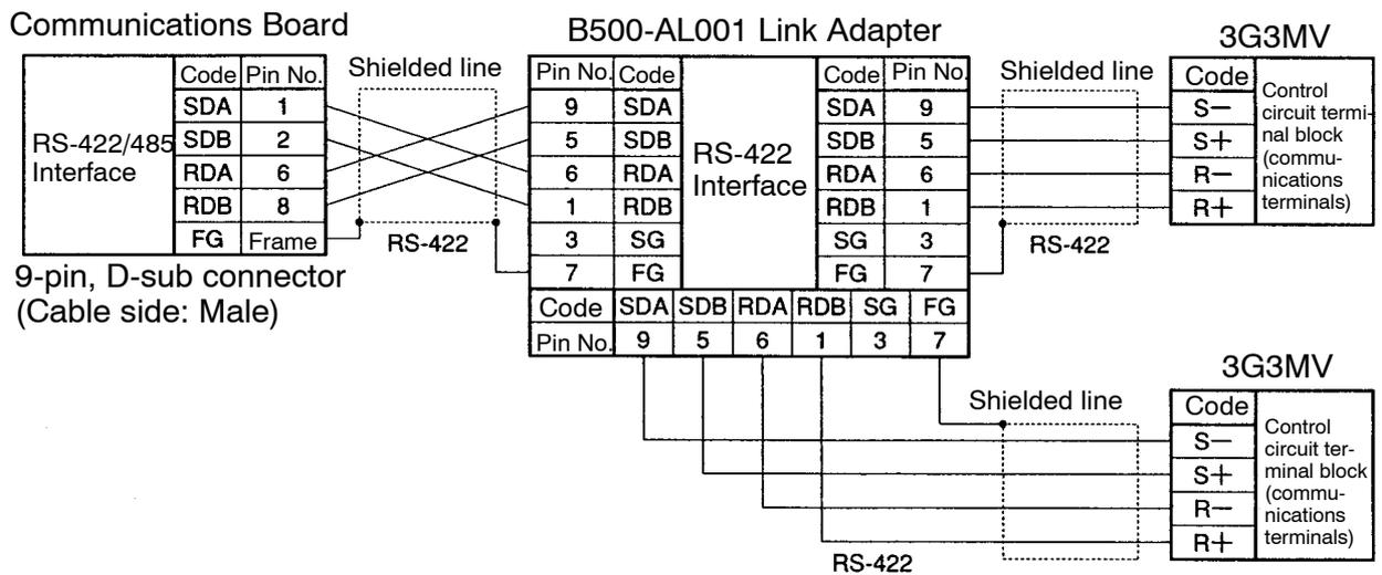
**Note** Turn the terminal resistance of all the Inverters to ON for RS-422 communications. Refer to page 2-18, *Selecting RS-422/485 Termination Resistance* for details.
