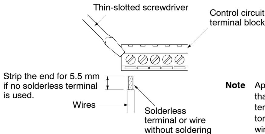
**Note** Applying a torque of greater than 0.5 N•m may damage the terminal block. If the tightening torque is insufficient, however, wires may be disconnected.
