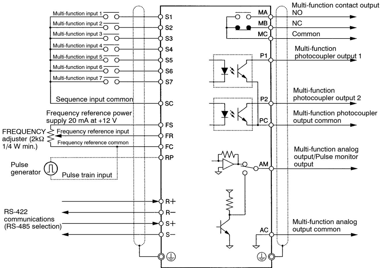
**Note** I/O signals can be connected to a single shielded cable.
