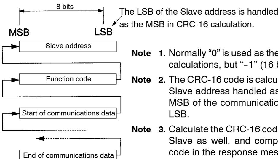
**Note 1.** Normally “0” is used as the initial value for CRC-16 calculations, but “-1” (16 bits all “1”) is used here.
