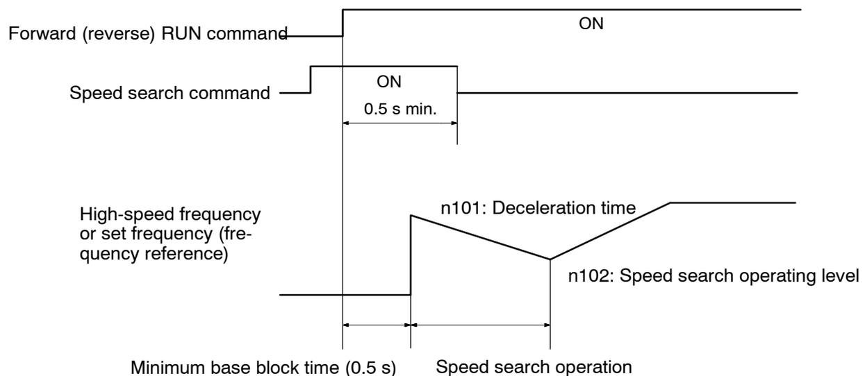
**Note** For 5.5- and 7.5-kW Inverters only, the speed search function can be adjusted by setting parameters n101 (speed search deceleration time) and n102 (speed search operating level). If the speed search cannot be executed properly using the default setting, lengthen the deceleration time or lower the operating level. To reduce the speed search time, check with the application while either shortening the deceleration time or raising the operating level.
