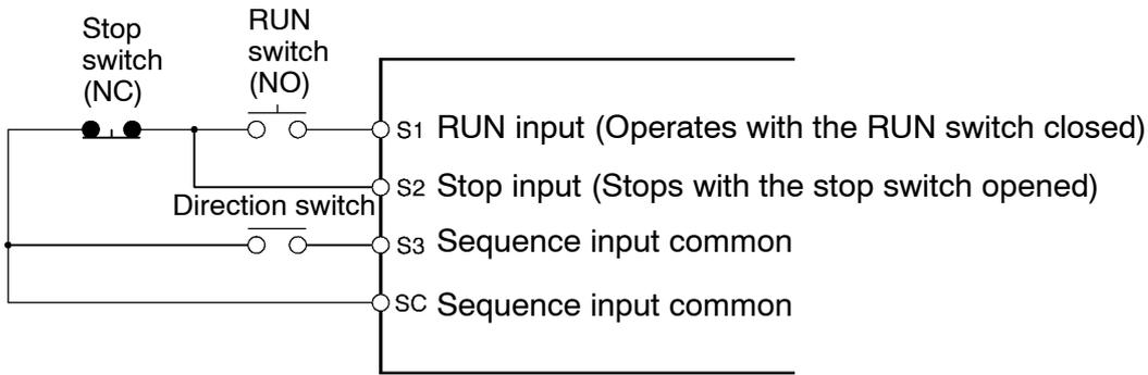
**Note** Set parameter 052 to forward/reverse rotation command 0 for 3-wire sequence input.
