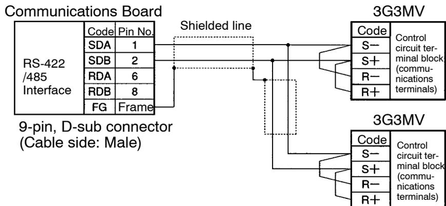
**Note** Be sure to set the terminal resistance of only the Inverter at each end to ON and that any other Inverter to OFF. Refer to page 2-18, *Selecting RS-422/485 Termination Resistance* for details.
