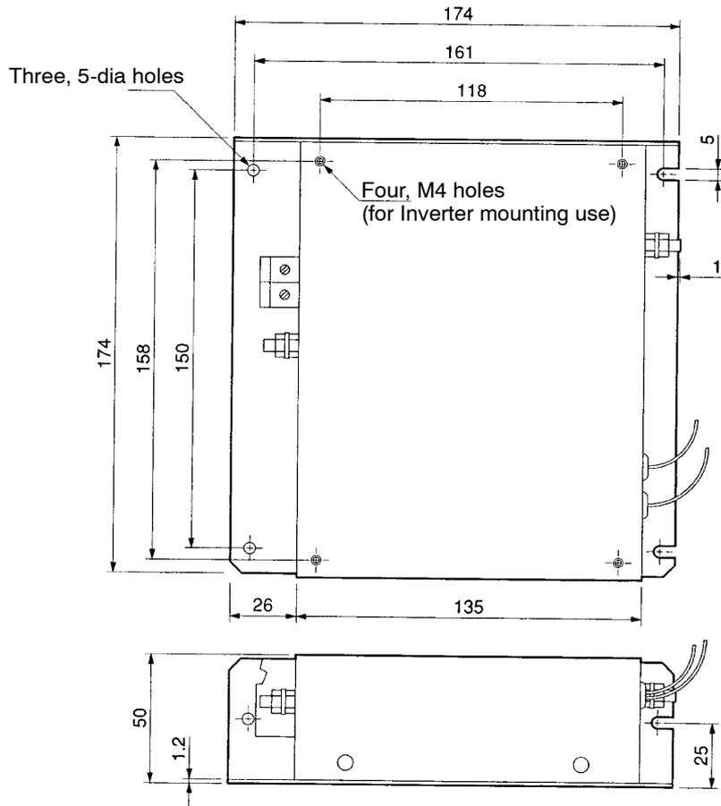
Noise Filters for 3-phase 200-VAC Inverter Models
