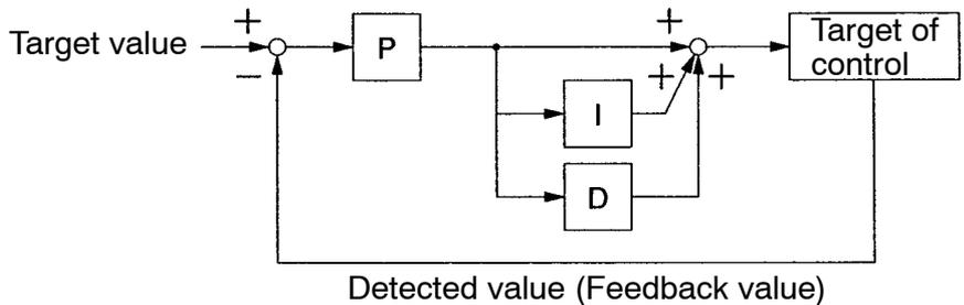
• Furthermore, 3G3MV Inverter can add the frequency reference to the operation result of the PID control block.
