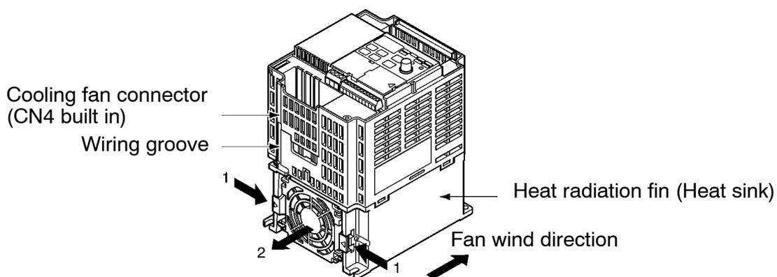
2. Press the left and right sides of the fan cover located on the lower part of the radiation fin in the arrow 1 directions. Then lift the bottom of the Fan in the arrow 2 direction to remove the fan as shown in the following illustration.
