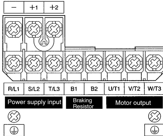
**Note** For single-phase input, connect R/L1 and S/L2.
