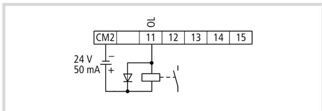
Figure 105: Digital output 11 configured as OL/OL2 (overload signal)
