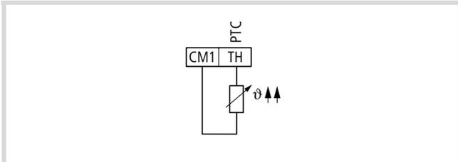
Figure 73: Connection, terminal TH
