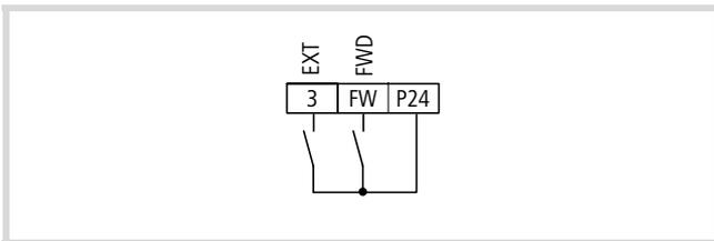
Figure 64: Digital input configured as FW (start/stop clockwise operation) and digital input 3 as EXT (external fault)
