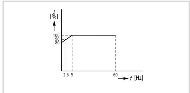
Figure 155: Normal overload protection (PNU b013 = 01)
