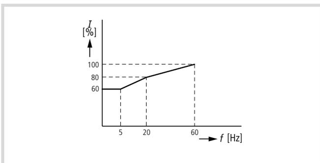
Figure 154: Increased overload protection (PNU b013 = 00)
