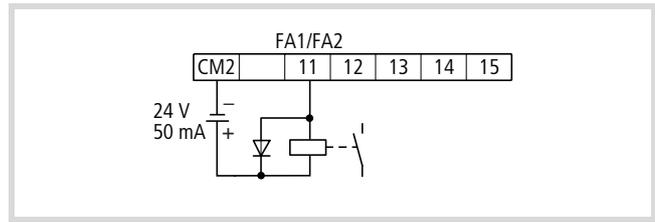
Figure 100: Digital output 11 configured as FA1/FA2 (frequency reached/exceeded)
