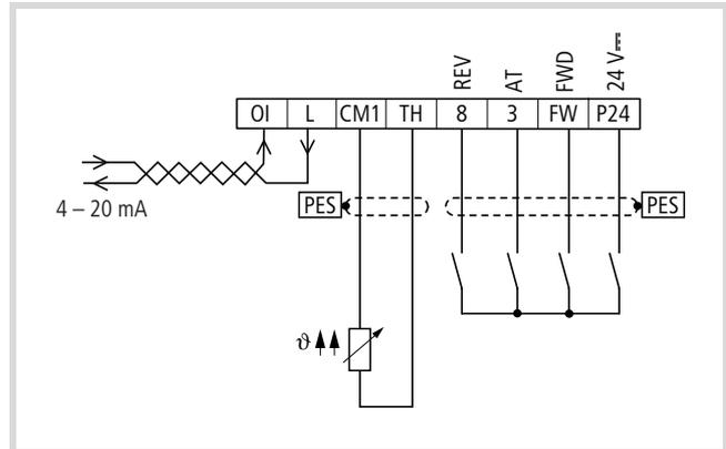
Figure 45: Analog setpoint definition
