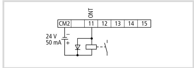
Figure 118: Digital output 11 configured as ONT (Mains On time)
