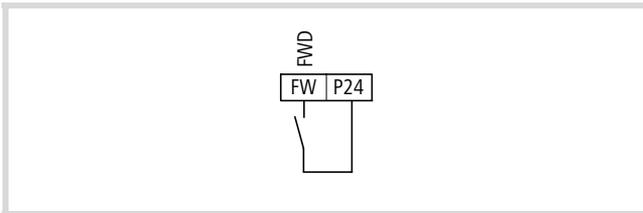
Figure 53: Digital input FW (start/stop clockwise)
