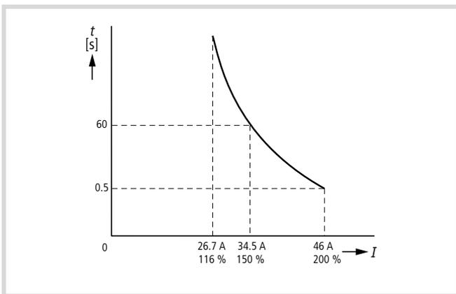
Figure 153: Tripping current characteristic at  $I_e = 23$  A
