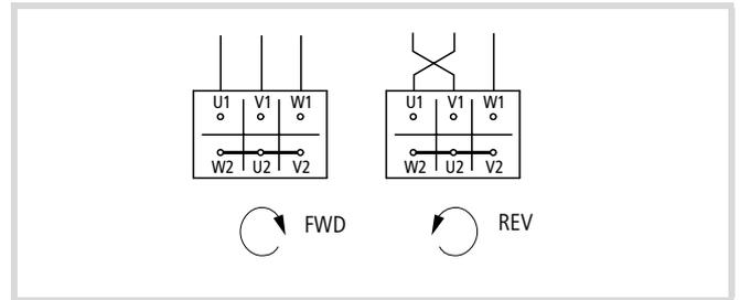
Figure 30: Direction of rotation, change of direction
