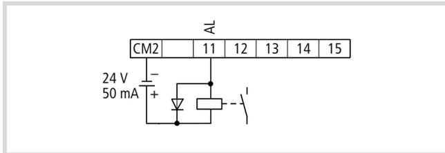
Figure 109: Digital output 11 configured as AL (fault occurrence)
