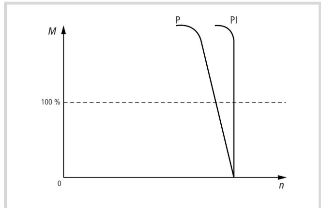
Figure 93: Function chart for PI and P control
