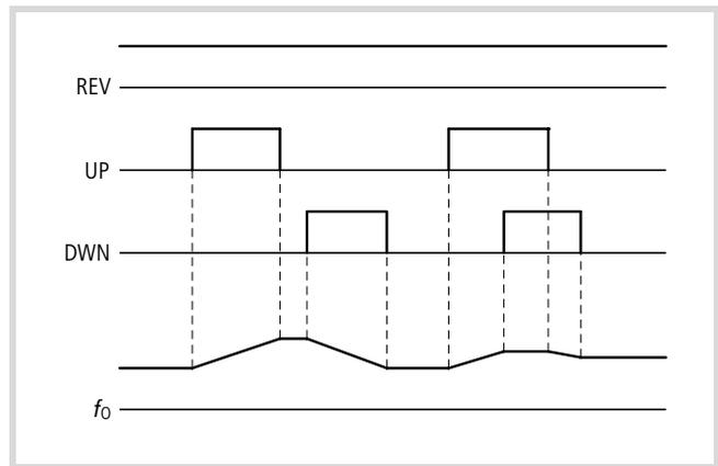
Figure 76: Function chart for UP/DWN (acceleration/deceleration – motor potentiometer)
