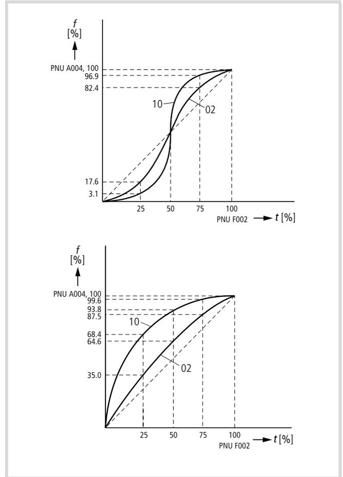
Figure 148: Curvature of the S- and U-curve characteristics
