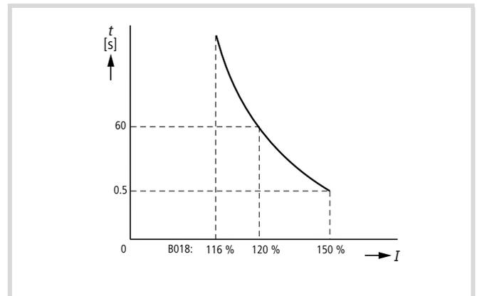
Figure 160: Tripping characteristic for adjustable overload protection using PNU b018
