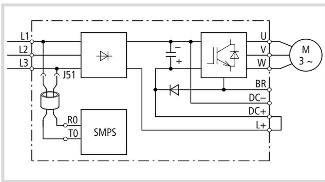
Figure 162: Default connection of terminals R0 and T0
