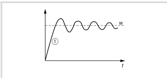
Figure 137: Oscillation, dampened
