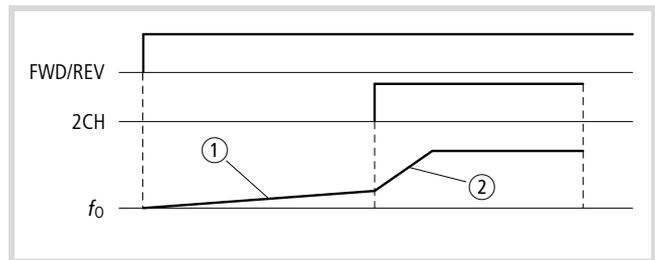
Figure 61: Function chart for 2CH (second acceleration time)
