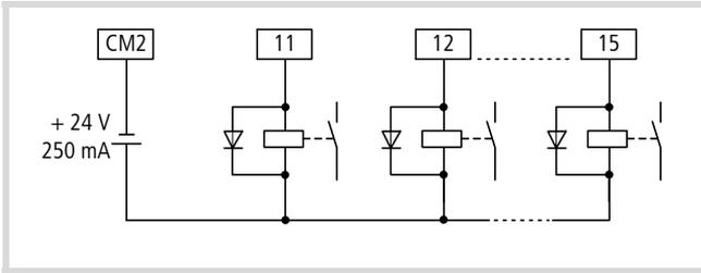
Figure 35: Relay with free-wheel diode
