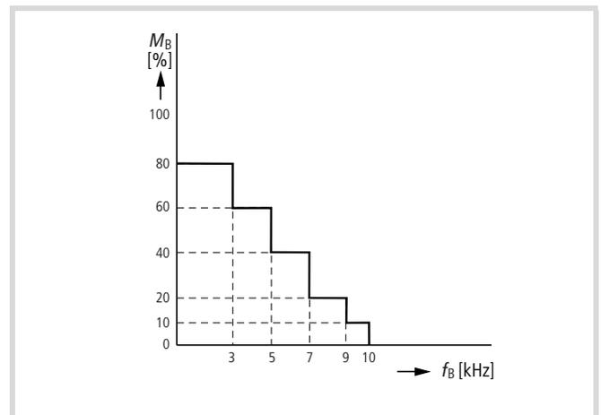
Figure 129: Derating for DC braking
