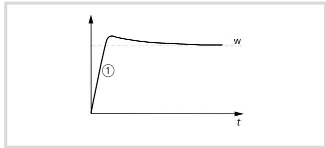
Figure 138: Good control characteristics
