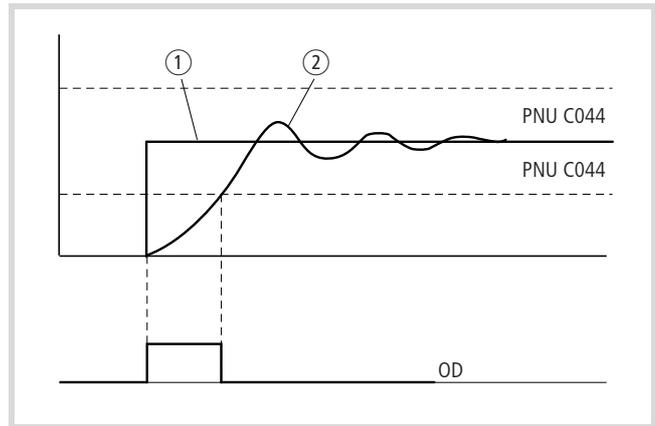
Figure 108: Function chart for OD (PID control deviation)
