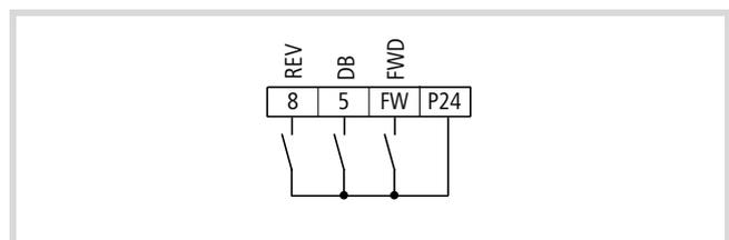
Figure 78: Digital input FW configured as FWD (start/stop clockwise operation), 8 as REV (start/stop anticlockwise operation), and 5 as DB (DC braking)
