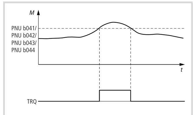
Figure 115: Function chart for TRQ (torque limitation)
