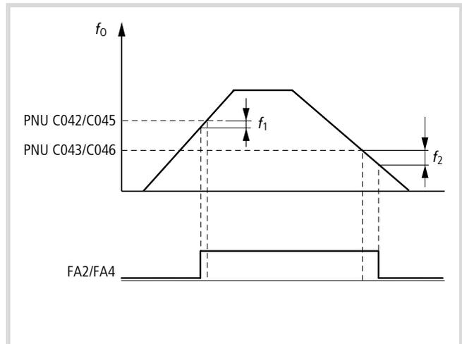
Figure 101: Function chart for FA2 (frequency exceeded)/FA4
