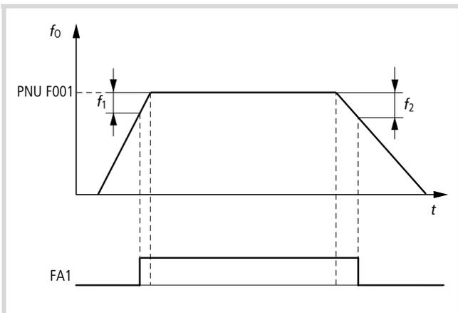
Figure 99: Function chart for FA1 (frequency reached)
