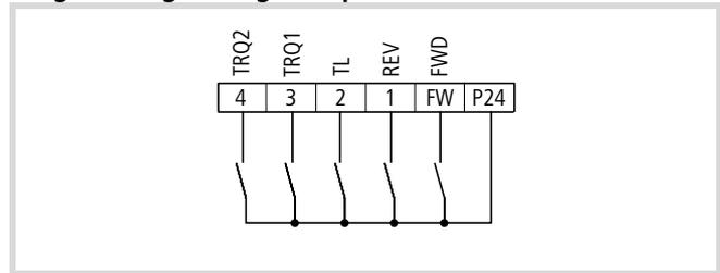
Figure 87: Digital input 1 configured as REV (start/stop anticlockwise operation), 2 as TL (activate torque limitation), 3 and 4 as TRQ1 and TRQ2 (bitwise selection of torque limits).
