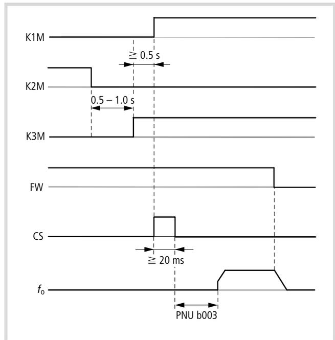
Figure 83: Function chart for CS (heavy mains starting)
