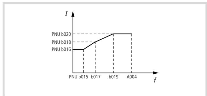
Figure 156: Adjustable overload protection (PNU b013 = 02)
