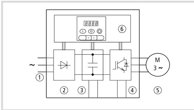
Figure 5: Function chart of the frequency inverter
