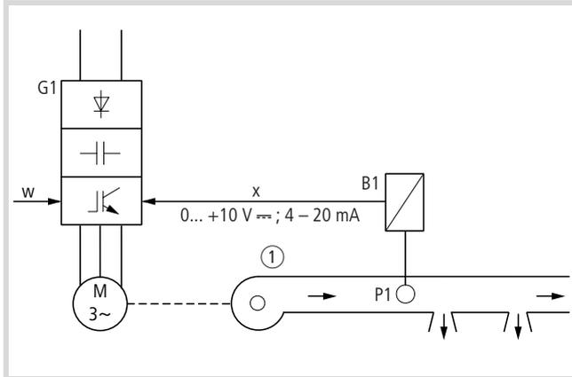
Figure 134: Example of a fan control system
