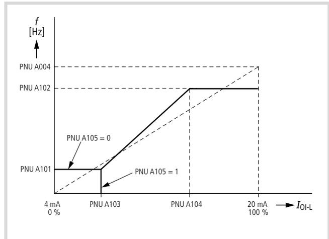
Figure 51: Setpoint current, terminals OI-L
