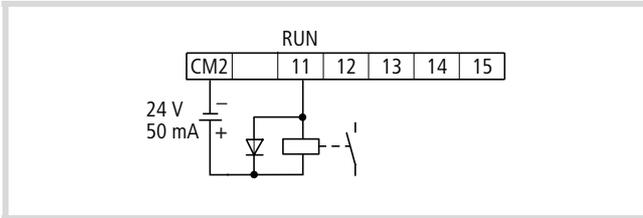
Figure 103: Digital output 11 configured as RUN (Run signal)
