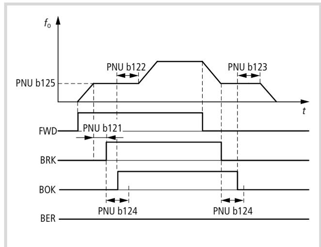
Figure 171: Brake control function chart
