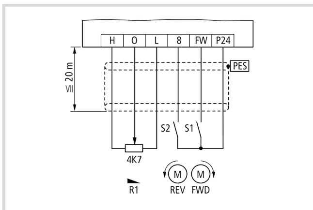
Figure 39: Connecting the control signal terminals (default settings)
