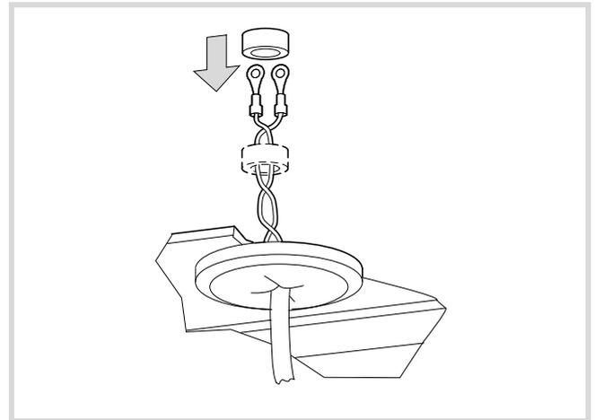
Figure 24: Push on the ferrite rings
