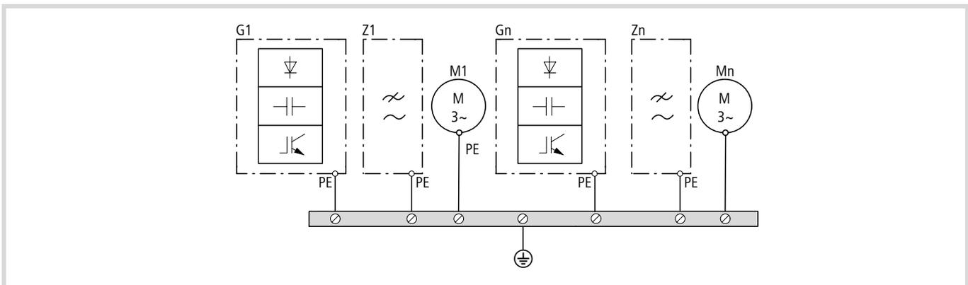
Figure 14: Star-type point-to-point earthing
