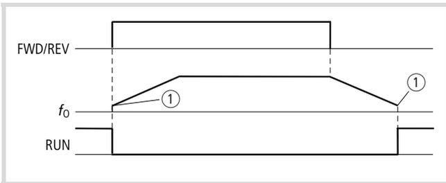
Figure 104: Function chart for RUN (Run signal)
