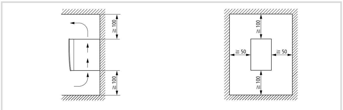
Figure 7: Installation dimensions
