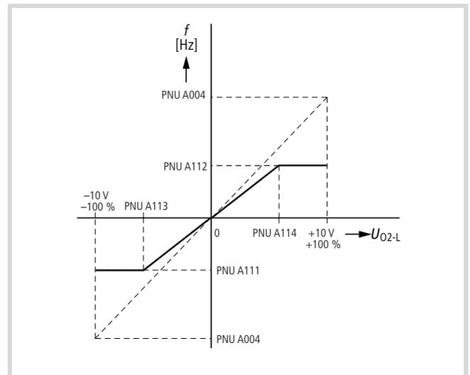
Figure 52: Setpoint matching, terminals O2-L
