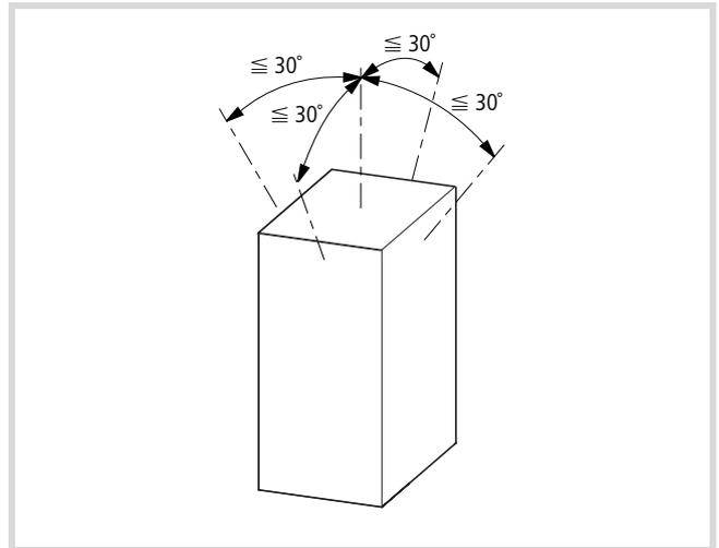
Figure 6: Mounting position
