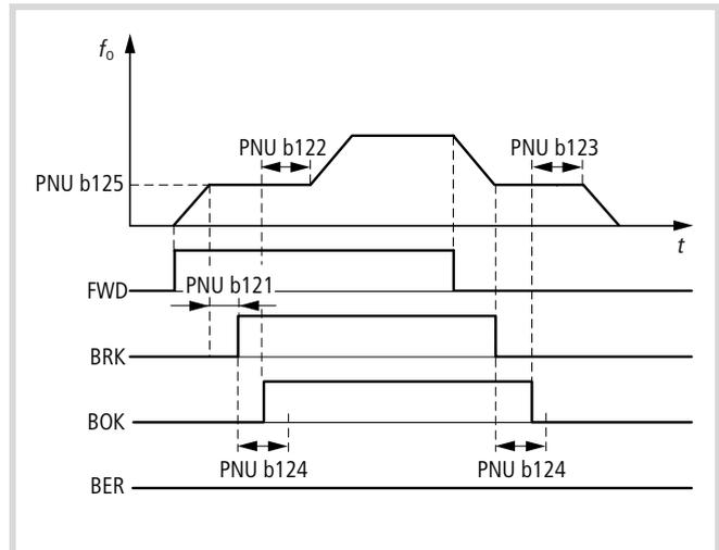
Figure 111: Brake control function chart
