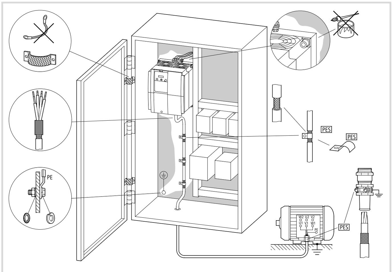
Figure 13: EMC-compliant setup
