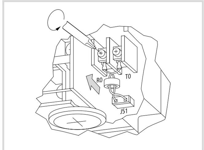
Figure 164: Disconnect J51 from terminals R0 and T0
