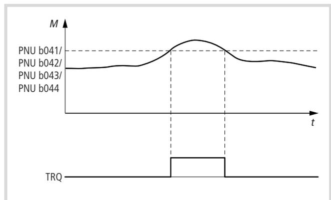
Figure 88: Function chart for torque limits
