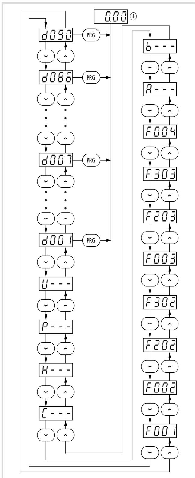
Figure 41: DV6 keypad menu structure
