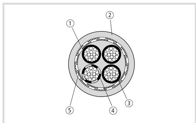
Figure 15: Sample motor cable
