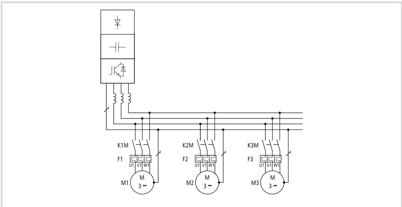
Figure 31: Parallel connection of multiple motors
