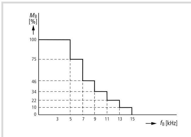
Figure 128: Derating for DC braking
