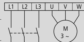
The arrangement of the power terminals is shown in the figure below.
