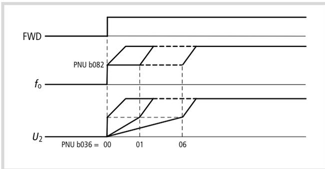
Figure 167: Function chart for voltage ramp reduction
