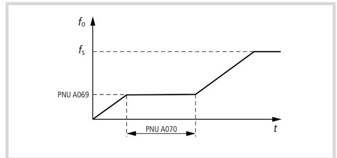
Figure 132: Function chart for acceleration waiting time
