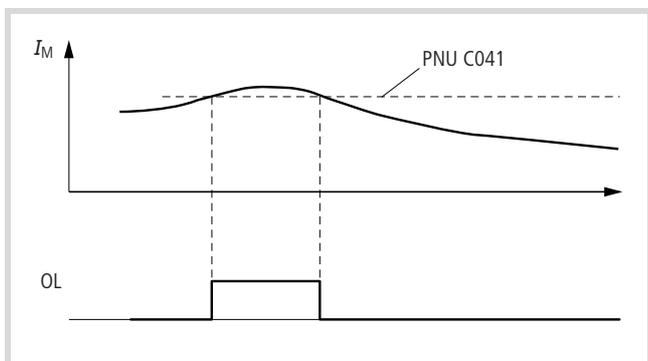
Figure 106: Function chart for OL (overload signal)/OL2
