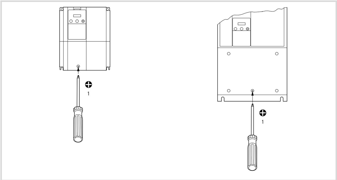
Figure 19: Loosening the screw
