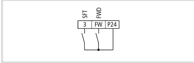
Figure 74: Digital input 3 configured as SFT (software protection)
