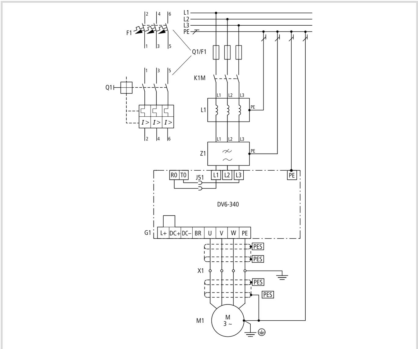
Figure 26: Power terminal connection
