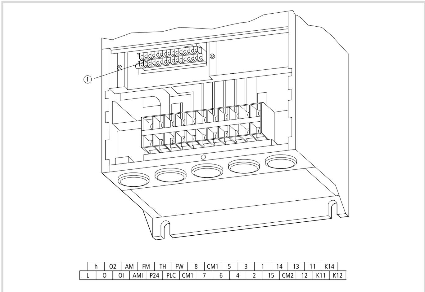
Figure 33: Location of the control signal terminals
