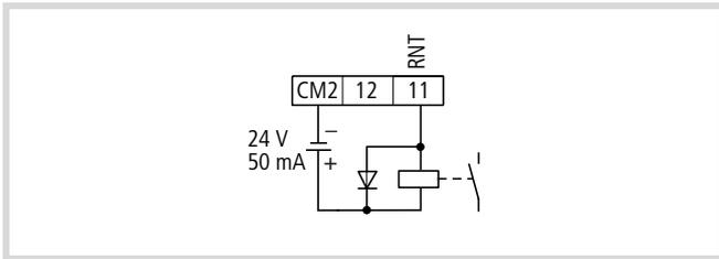
Figure 116: Digital output 11 configured as RNT (running time)
