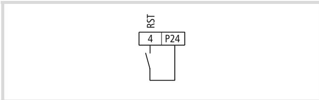
Figure 68: Digital input 4 configured as RST (reset)
