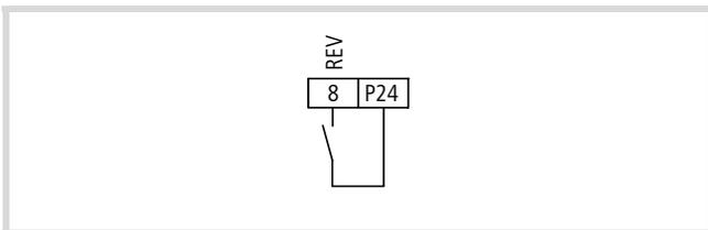
Figure 54: Digital input 8 configured as REV (start/stop anticlockwise)
