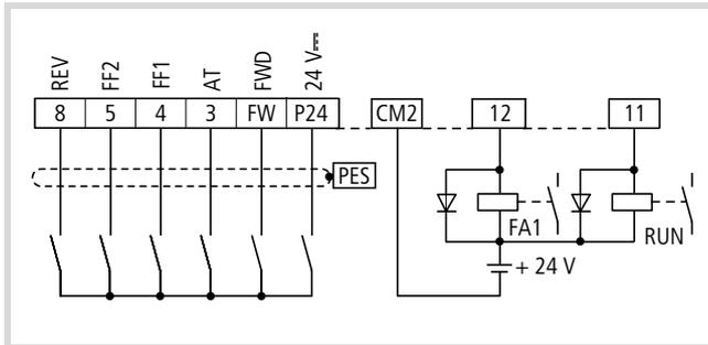
Figure 46: Fixed frequency definition
