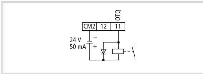
Figure 112: Digital output 11 configured as OTQ (torque exceeded)
