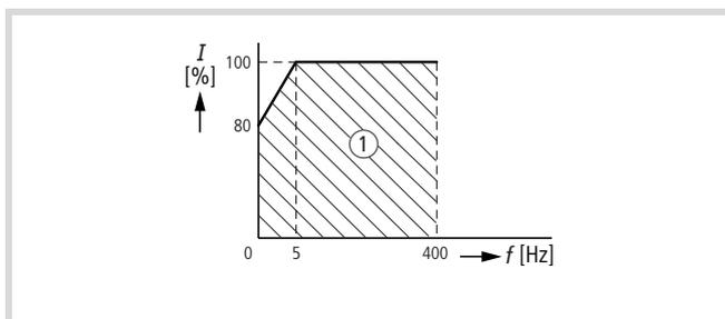
Figure 159: Setting range for the adjustable overload protection
