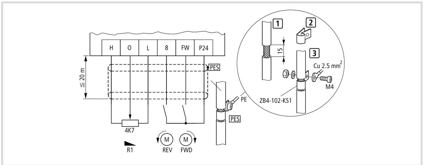
Figure 34: Control terminal connection (factory setting)
