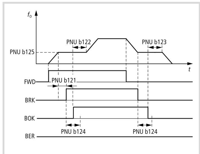
Figure 97: Brake control function chart
