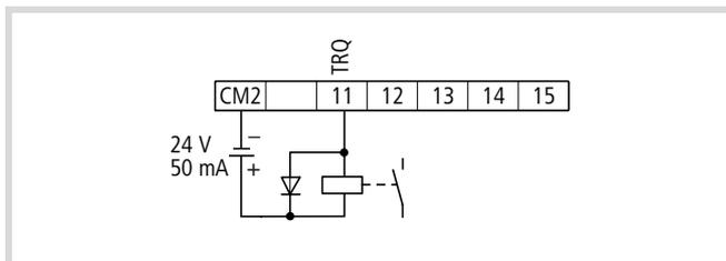
Figure 114: Digital output 11 configured as TRQ (torque limitation).
