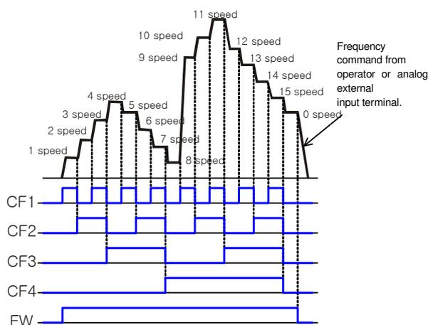
Example) The setting method for Multi-speed operation from control terminals
