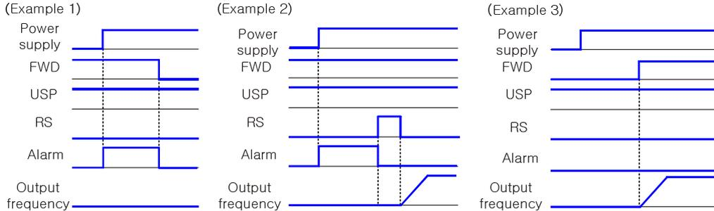
Example) In case Assign 13[USP] to an input terminal (DI2)
