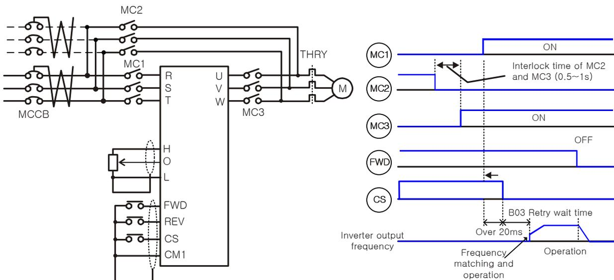
Example) Assigning 12[CS] to an intelligent input terminal [DI2].
