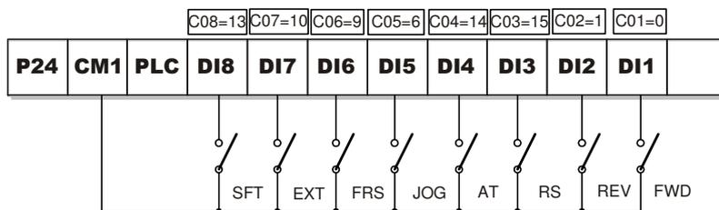
Example) FWD command on DI1 terminal, Setting D12~D15 to Multi-speed CF1~CF4 :
