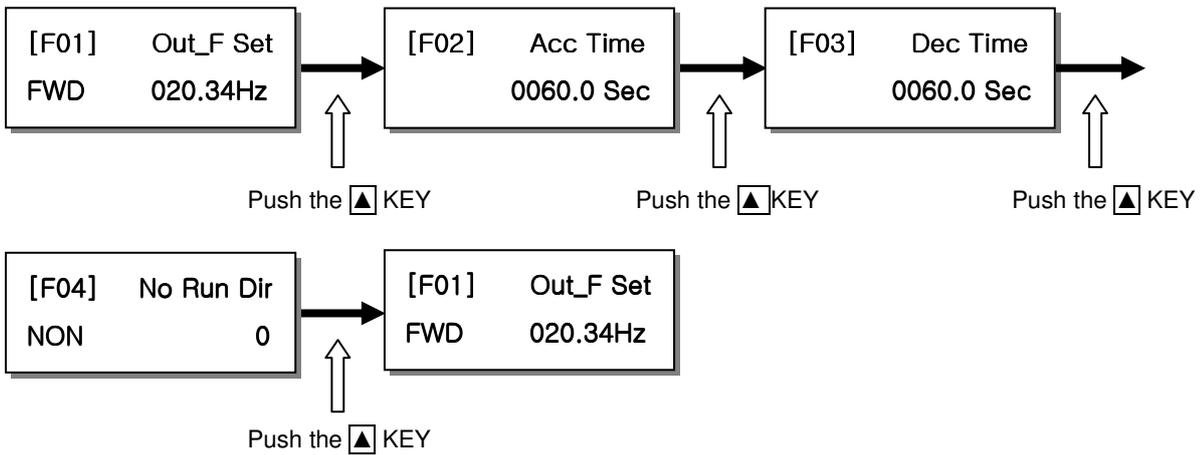
2) Setting method of parameter value (Example: Change of frequency parameter)
