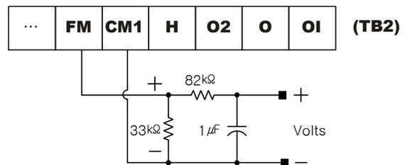
**Analog output signal (AM/AM2) Selection (C34~C35)**
