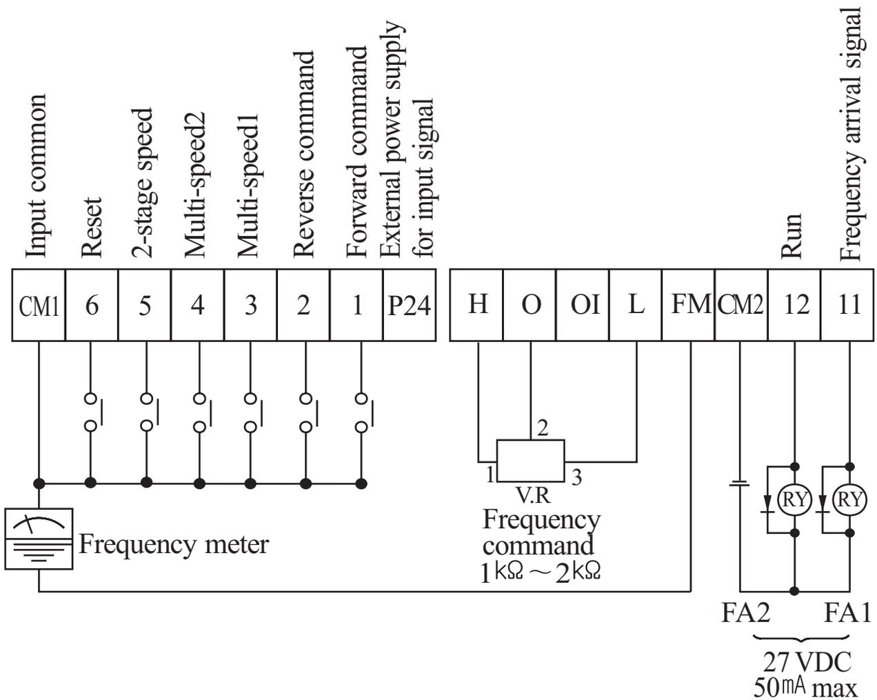
**Note1)** When an output intelligent terminal is used, be sure to install a surge absorbing diode in parallel with relay. Otherwise, the surge voltage created when the relay goes ON or OFF may damage the output intelligent terminal circuit.
