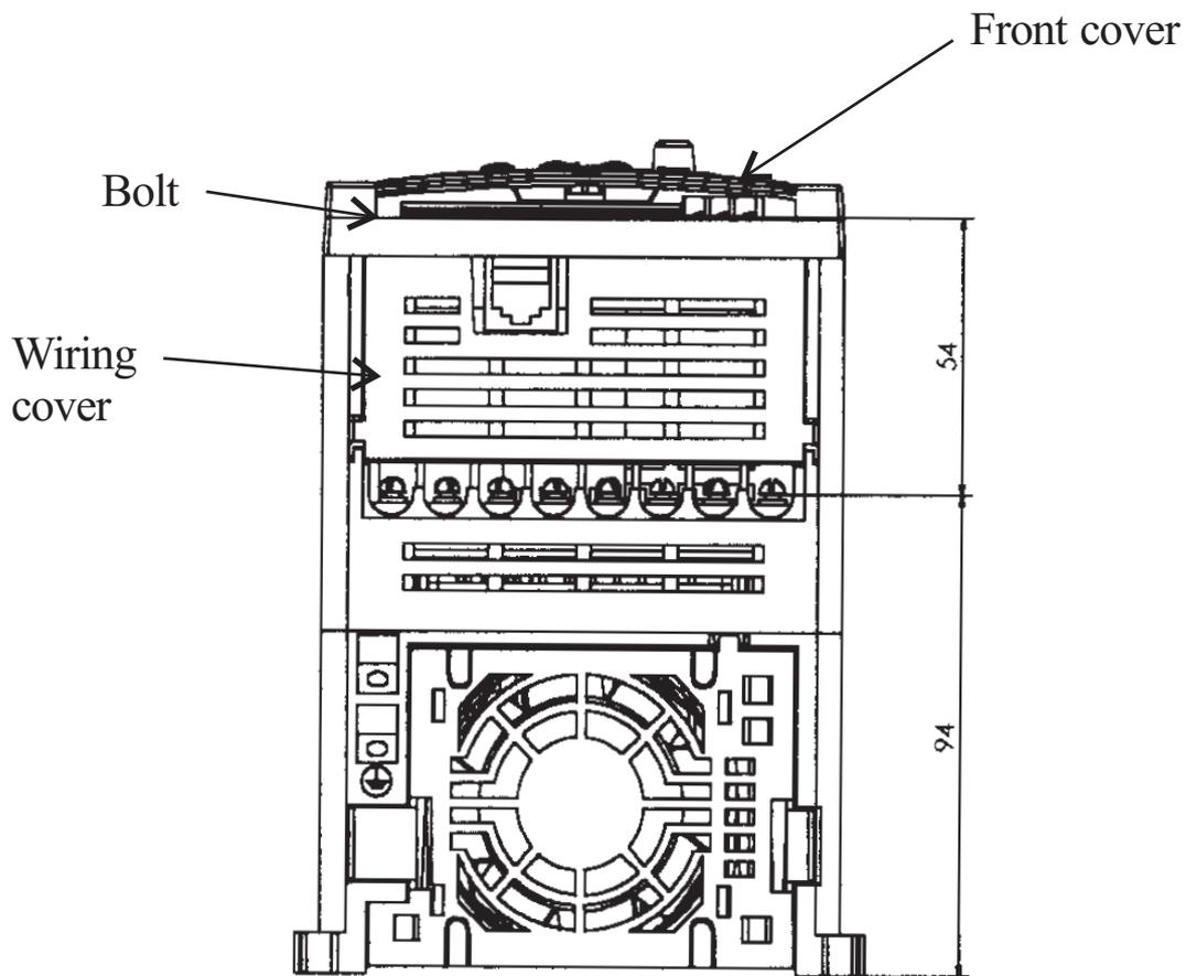
Use a screwdriver to loosen the Bolt on the front cover.
