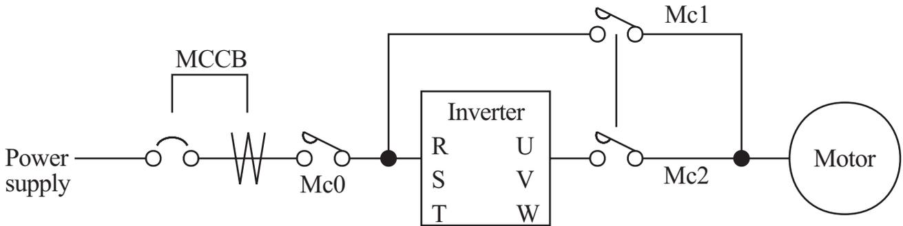
**NOTE2)** Install an earth leakage breaker(or MCCB) on the power supply side of the inverter. If the wiring distance between inverter and motor (10m and more) is long, the thermal relay may be incorrectly operated on the effect of high-frequency noise. Install the AC reactor on the inverter output side or use the current sensor.
