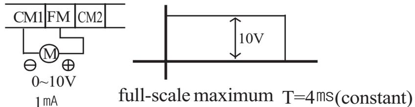
Note) This is dedicated indicator, so that it cannot be used as a line speed signal. The indicator accuracy after adjustment is about  $\pm 5\%$  (Depending on the meter, the accuracy may exceed this value)
