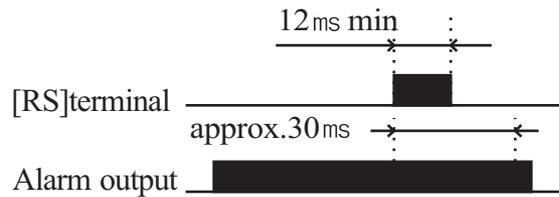
The input timing requirement for [RST] needs a 12 ms pulse width or greater. The alarm output will be cleared within 30 ms after the onset of the Reset command.
