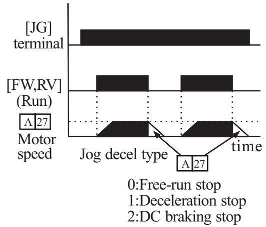
The type of deceleration used to end a motor jog is selectable by programming function **A27**. The options are:
