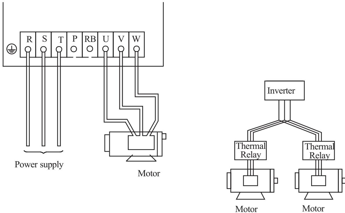
Always connect the power input terminals R, S, and T to the power supply.
