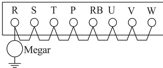
Never test the withstand voltage on the inverter. The inverter has a surge protector between the main circuit terminals and the chassis ground.
