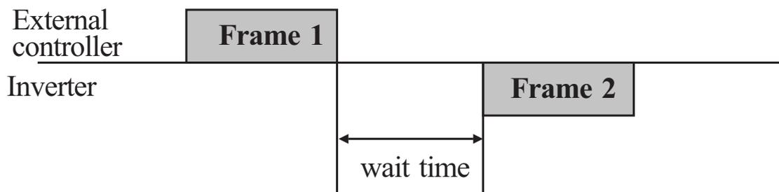
Frame start : Frame start is recognized by signal line data transmitted.
