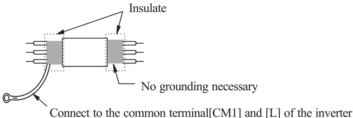
**Note3)** When the frequency setting signal is turned on and off with a contact, use a relay which will not cause contact malfunctions, even with the extremely weak currents and voltages.
