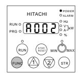
The changed set value is confirmed by pushing the STR key.
