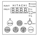
Hold down the FUNC, UP and DOWN key and then press the STR key. When the display starts to flash and rotate release all the keys.
