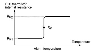
Suppose that the internal resistance of the PTC thermistor at the alarm temperature is Rp, the detection level (voltage)  $V_{v2}$  is calculated by the expression below. Set the result  $V_{v2}$  to function code H27.
