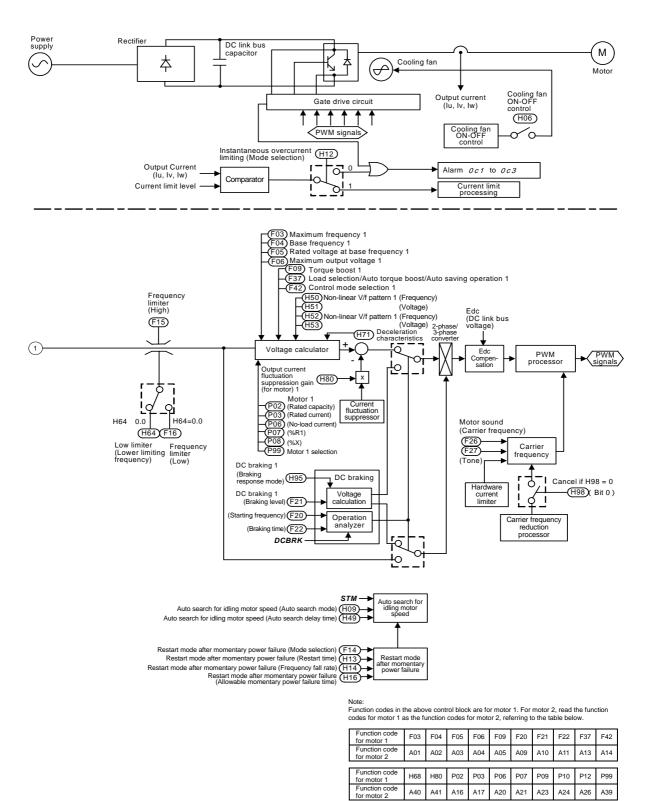
Figure 4.3.2 Control Block -- Output Stage
