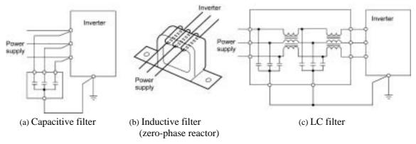
Figure A.10 Various Filters and their Connection
