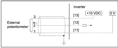
Figure 6.13 External Potentiometer Dimensions and Connection Example
