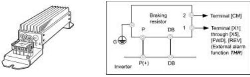
Figure 6.6 Braking Resistor (Standard Model) and Connection Example
