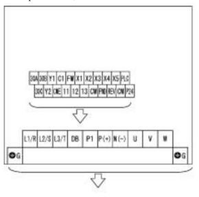
Three-phase 200 V, 5.5 to 7.5 kW Three-phase 400 V, 5.5 to 7.5 kW
