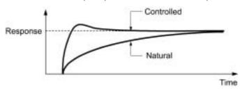
3) Suppressing oscillation whose period is longer than the integral time specified by J04 Increase the data of J04 (Integral time).
