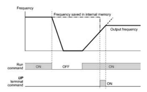
Initial frequency for the *UP/DOWN* control when the frequency command source is switched When the frequency command source is switched to the *UP/DOWN* control from other sources, the initial frequency for the *UP/DOWN* control is as listed below:
