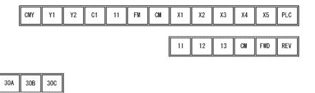
Screw size: M3, Tightening torque: 0.5 to 0.6 (N·m)
