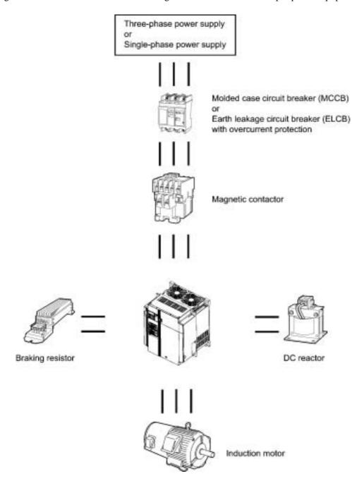
Figure 1.25 Recommended Configuration Diagram
