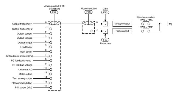
Figure 4.6 Terminal [FM] Output Selector
