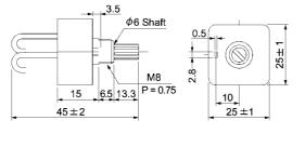
Dial plate type: YS549810-0 Knob type: MSS-2SB  $\frac{1-\phi 5}{50}$ FREO SET  $\frac{1}{40}$   $\frac{\phi 3.2}{1-\phi 10}$ Unit: mm
