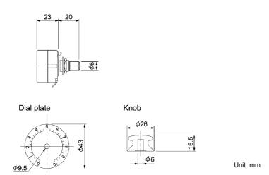
Note: The dial plate and knob are supplied together with the external potentiometer WAR3W. Available from Fuji Electric Technica Co., Ltd.
