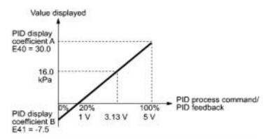
■ Display coefficients for PID dancer positioning command and its feedback (J01 = 3) Under the PID dancer control, the PID dancer positioning command and its feedback operate the range within  $\pm 100\%$ , so specify the value at +100% of the PID command or its feedback as coefficient A with E40, and the value at -100% as coefficient B with E41.
