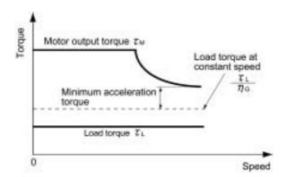
Figure 7.4 Example Study of Minimum Acceleration Torque
