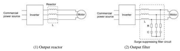
Figure C.3 Method to Suppress Surge Voltage
