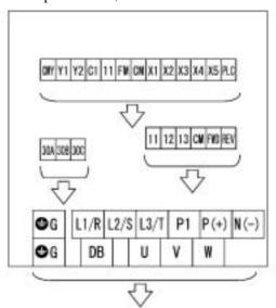
Three-phase 200 V, 1.5 to 3.7 kW Three-phase 400 V, 0.4 to 3.7 kW
