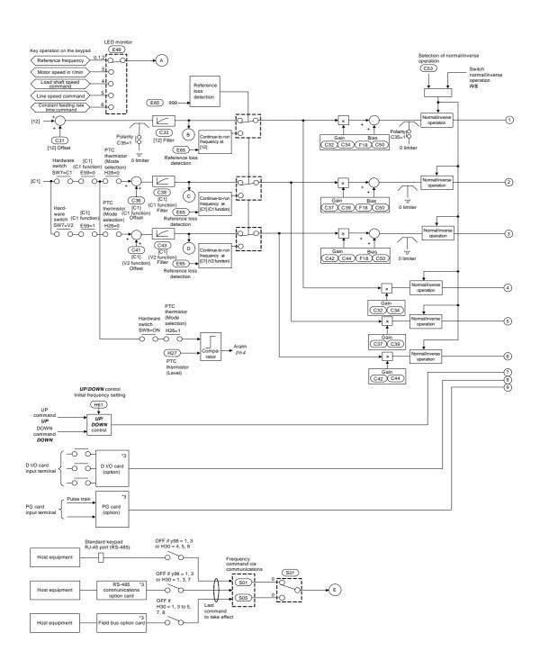
Figure 4.1.1 Drive Frequency Command Block -- Input Stage
