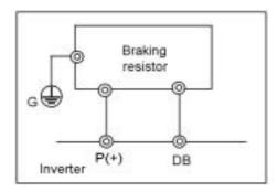
Figure 6.8 Braking Resistor (Compact Model) and Connection Example
