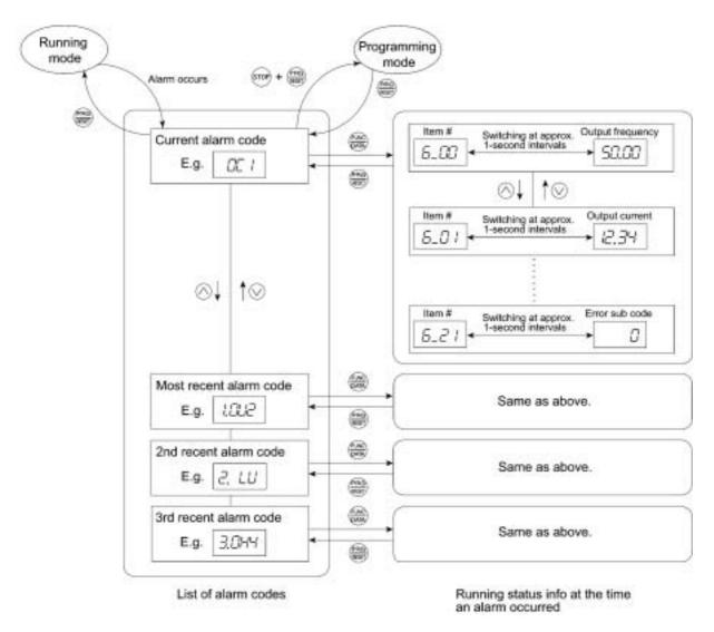
Figure 3.11 Menu Transition in Alarm Mode
