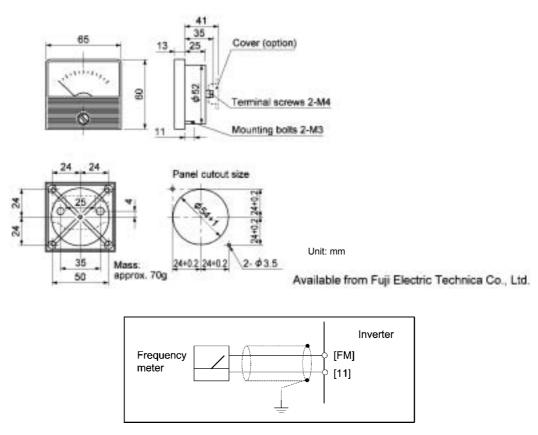
Figure 6.14 Frequency Meter Dimensions and Connection Example
