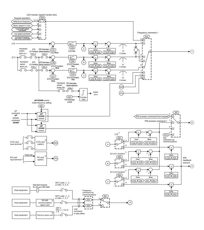
Figure 4.4.1 PID Process Control Block -- Input Stage
