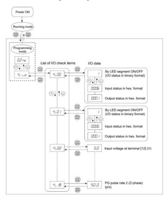
Figure 3.8 Menu Transition in Menu #4 "I/O Checking"
