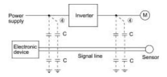
Figure A.5 Electrostatic Induced Noise
