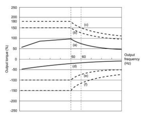
Figure 7.1 Output Torque Characteristics (Base frequency: 50 Hz)
