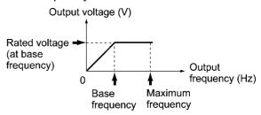
The minimum frequency at which an inverter delivers a constant voltage in the output V/f pattern. Related function codes: F04 and A02
