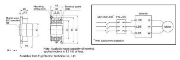
Figure 6.3 Dimensions of Surge Killer and Connection Example
