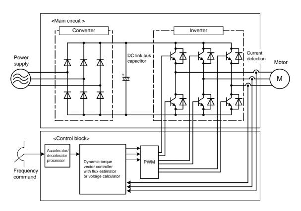
Figure 1.24 Schematic Overview Block Diagram of FRENIC-Multi
