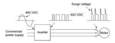
Figure C.1 Voltage Waveform of Individual Portions
