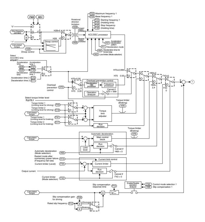
Figure 4.3.1 Control Block -- Input Stage
