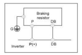
Figure 6.7 Braking Resistor (10%ED Model) and Connection Example
