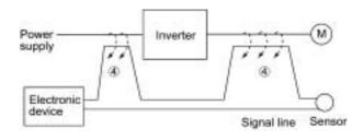
Figure A.4 Electromagnetic Induced Noise
