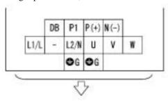
Three-phase 200 V, 1.5 to 2.2 kW Three-phase 400 V, 0.4 to 2.2 kW
