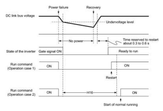
If H16 (Allowable momentary power failure time) is set to "999," restart will take place until the DC link bus voltage drops down to the allowable voltage for restart after a momentary power failure (50 V for 200 V class series and 100 V for 400 V class series). If the DC link bus voltage drops below the allowable voltage, the inverter recognizes that the power has been shut down so that it does not restart but starts (normal starting).
