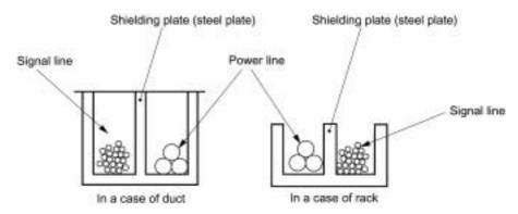
Figure A.7 Separate Wiring
