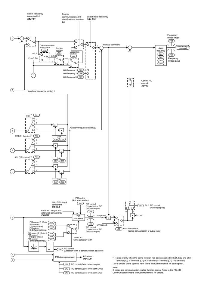
Figure 4.5.2 PID Dancer Control Block -- Output Stage
