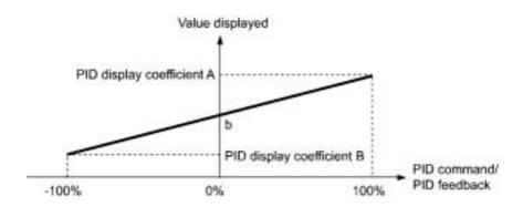
If the sensor output is unipolar, the PID dancer control operates within the range from 0 to +100%, so virtually specify the value at -100% as coefficient B.
