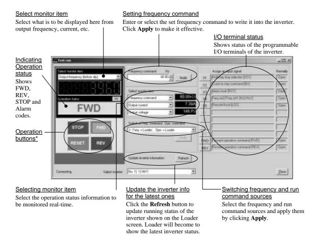
\* Refer to the table shown below for details of the operation buttons. The indented appearance of the **FWD** button as shown in the figure above indicates that it is active for running the motor forward, while that of the REV button is same for running reverse.
