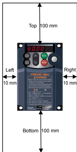
Figure 2.1 Mounting Direction and Required Clearances
